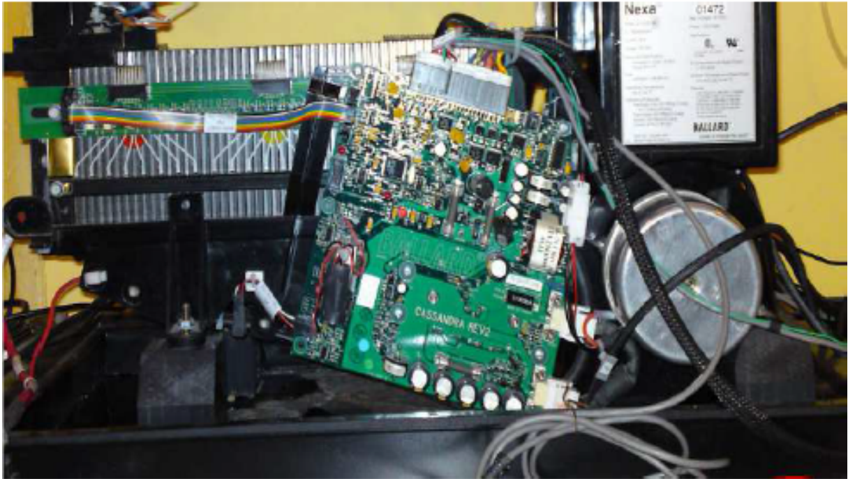
Fig 1.8: Pile PEM NEXA Ballard 1.2 KW.[SAA15]
