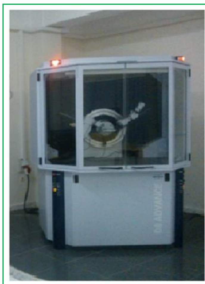
Figure III.4: Diffractomètre de type Bruker D8 Advance.
