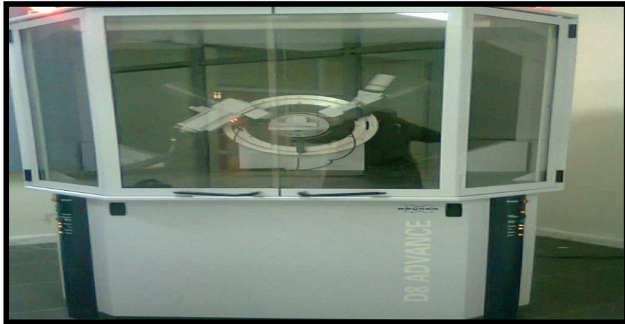
Figure II.7. BRUKER-AXS type D8 ADVANCE diffractometer.
