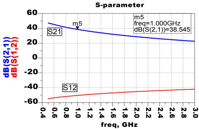
Figure.III.5: The performances of LNA (S-parameter). source common cascade
