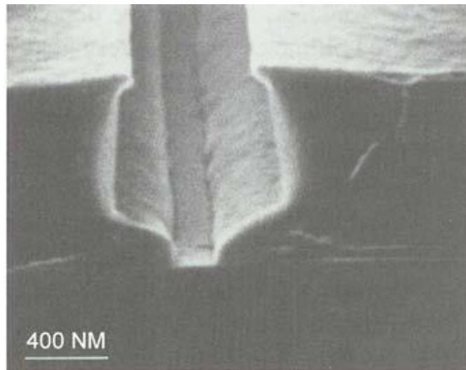
**Figure I.4:** T-shaped resist cavity using the trilayer resist system.
