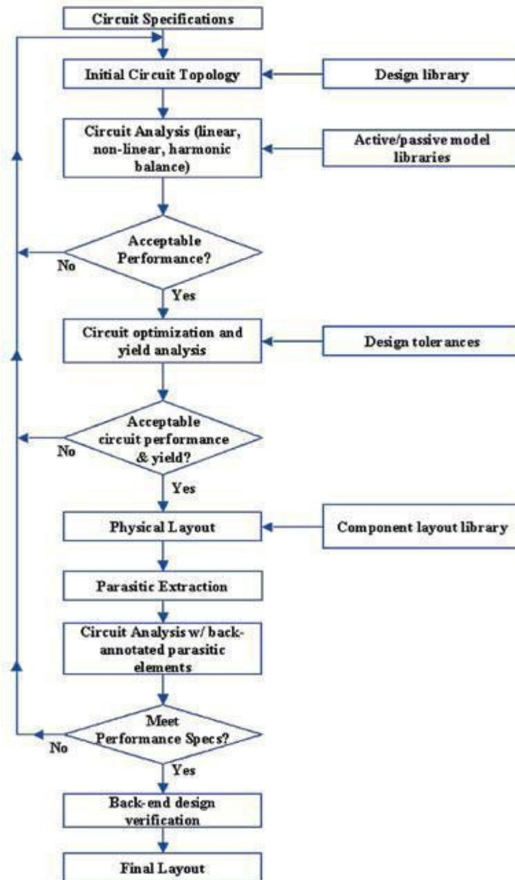
**Figure.II.2:** Typical MMIC design flow [5]
