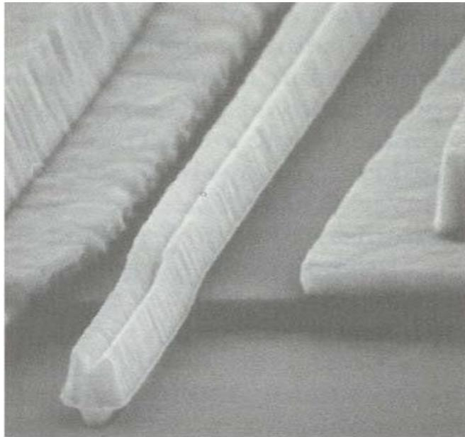
**Figure I.5:** T-shaped gate structure formed using the trilayer resist system.
