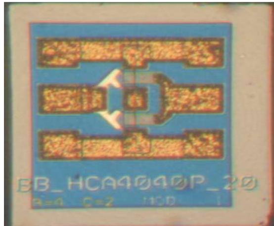
**Figure I.8:** Typical HEMT chip after scribe and break. (Note: all chips are inscribed with data identifying position on the wafer, gate number, and gate width [3].)
