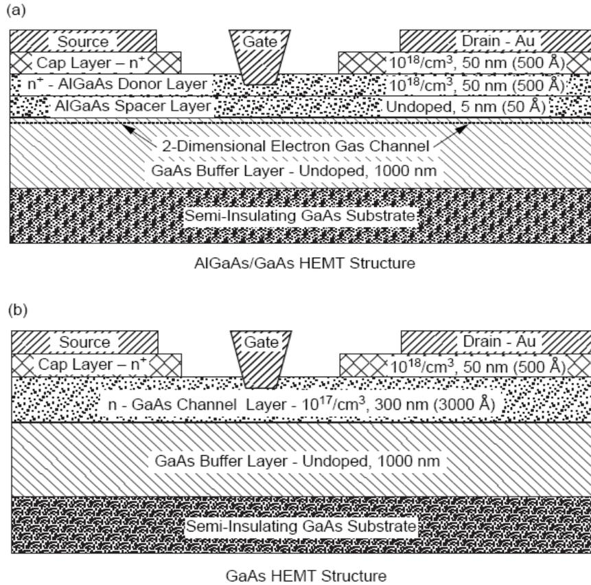
**Figure I.2:** Cross sectional diagrams comparing structures of an (a) AlGaAs/GaAs HEMT and a (b) GaAs MESFET [2].
