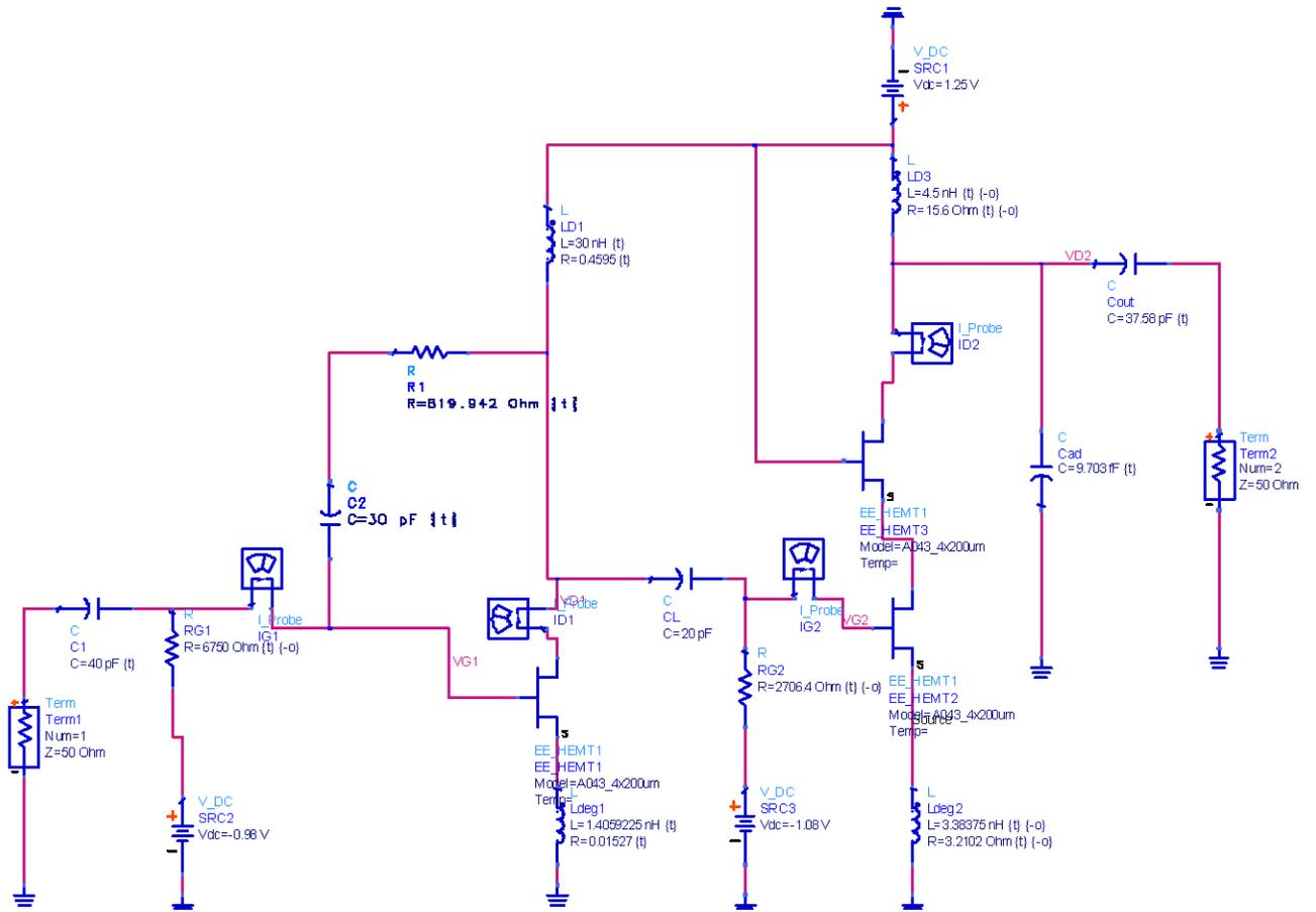
**Figure.III.3:** The amplifier LNA , Three-stages common source and cascode configuration
