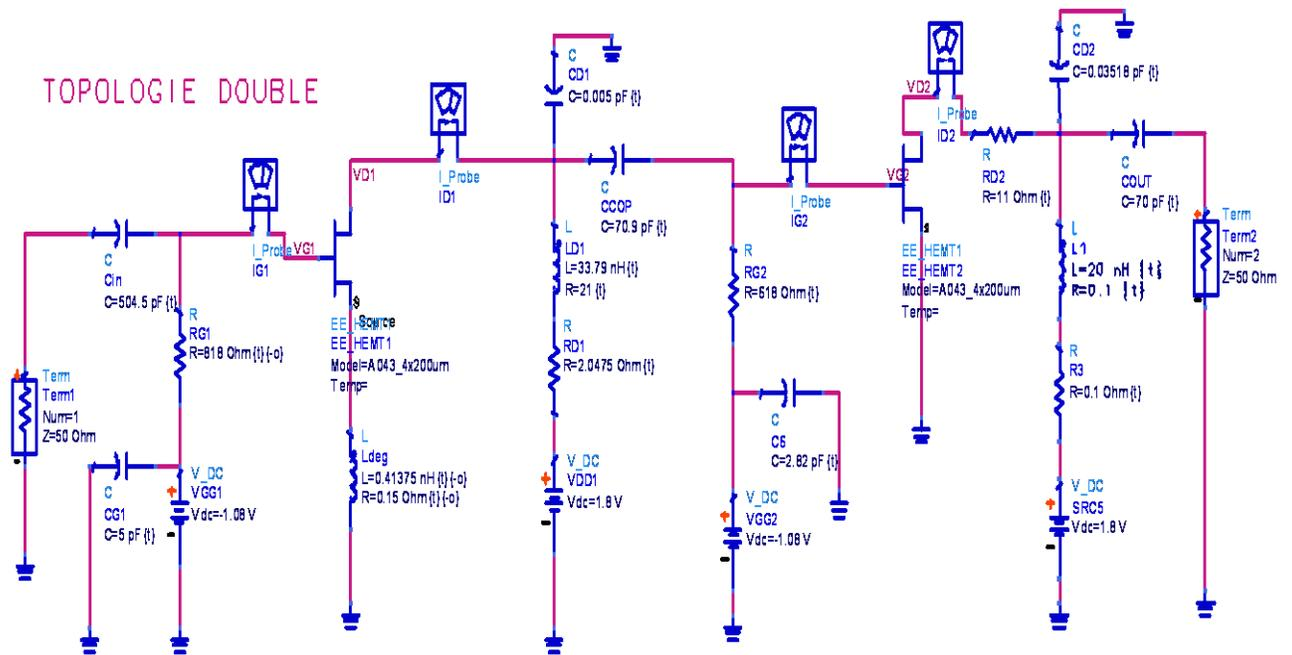
Figure III.2: circuit LNA, double stages common source cascaded.
