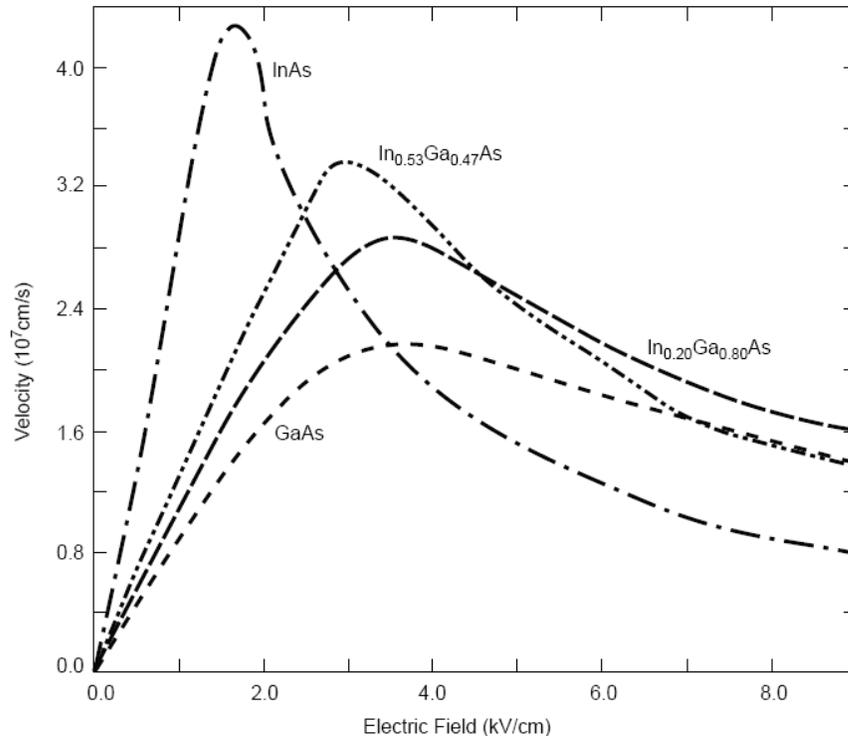
**Figure I.3:** Electron velocity as a function of electric field for variety of In concentrations of InGaAs.
