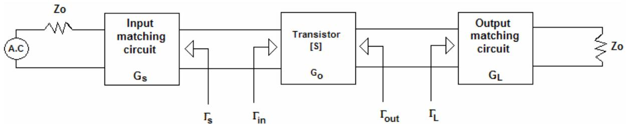
**Figure II.4:** Amplifier General Circuit.
