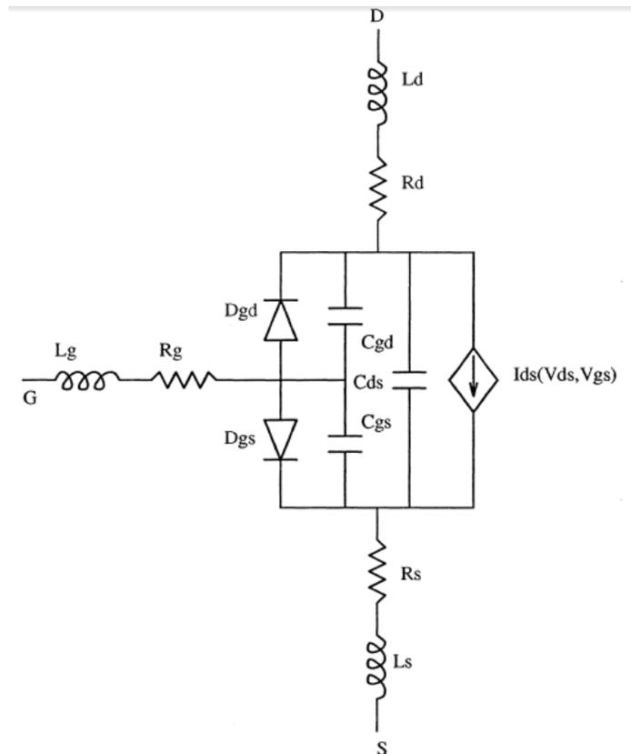
**Figure I.9:** The large signal model of a HEMT [11].
