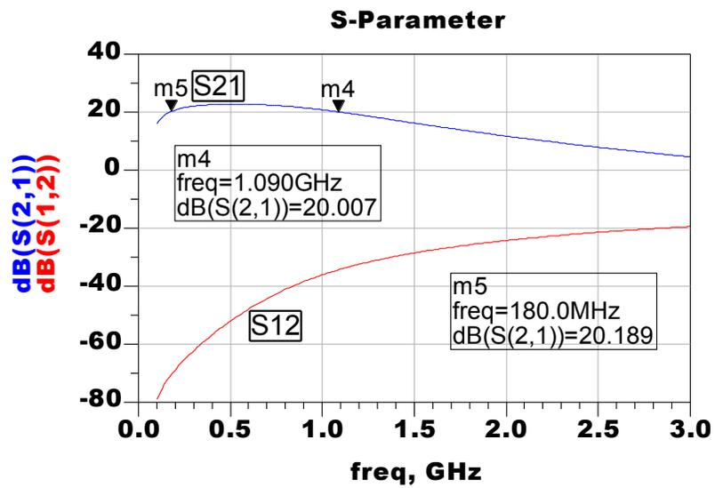
**Figure III.8:** The performances of LNA (S-parameter). source common three-stages cascode.
