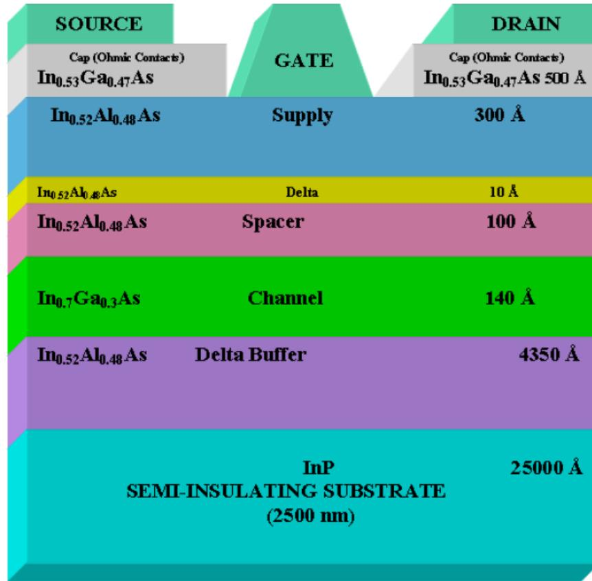
**Figure III.1:** The epitaxial layer structure of the pHEMT used in this work to design radio frequency LNAs [3].
