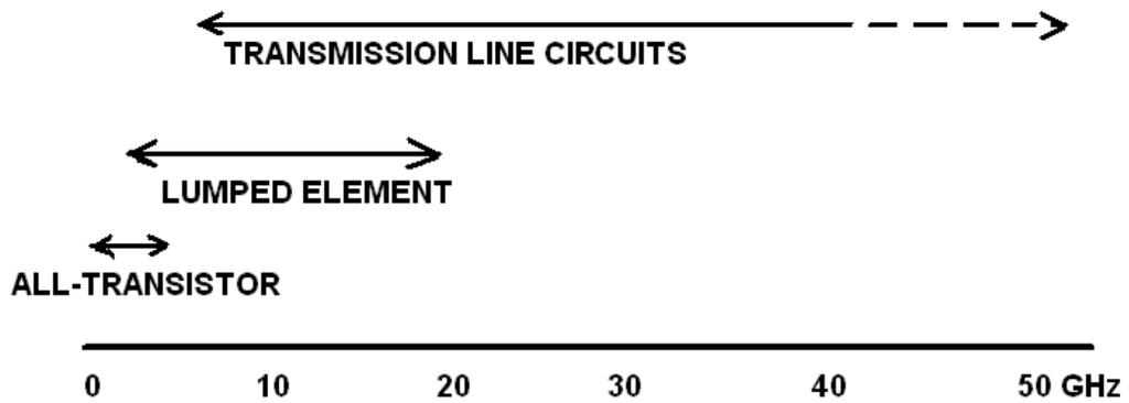
**Figure II.1:** Typical frequency range of operation for the three approaches of MMIC design.
