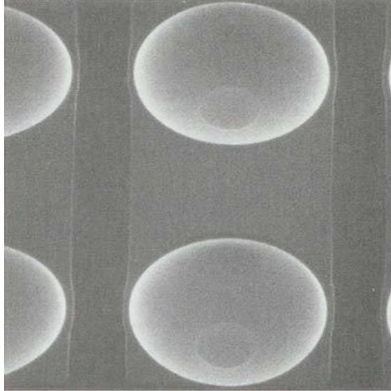
**Figure I.7:** Via-holes etched through a 4-mil-thick (10 $\mu$ m) GaAs substrate using a wet etch.
