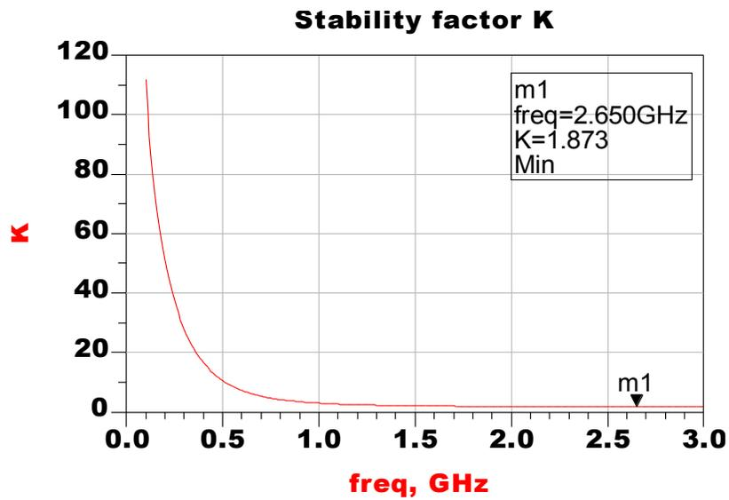
Figure III.7: (a) The stability of LNA cascode, (b) The noise factory.
