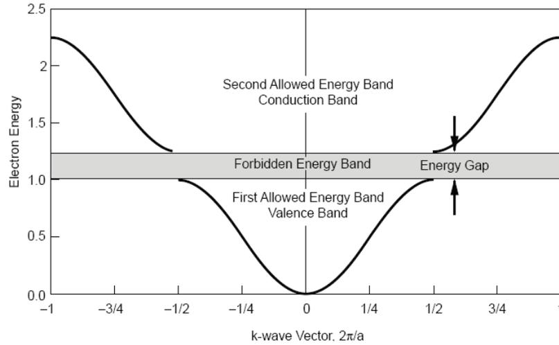
**Figure I.1:** Electron energy plotted as a function of wave-vector  $k$  ( $2\pi/a$ ) for an electron in a one-dimensional solid of lattice constant  $a$  showing the energy gap.
