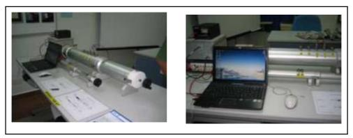
Figure 3.49: Impedance tube instrument and Configuration of Acoustic characteristics.
