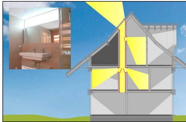
Figure 14: light pipe. (Source: www.energobal.ru )
