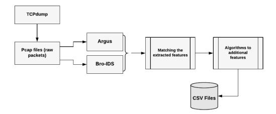
Figure 4.1: Framework Architecture for Generating UNSW-NB15 dataset
