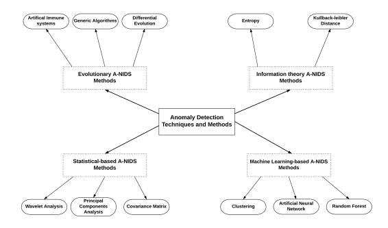
Figure 2.6: Anomaly detection techniques and methods
