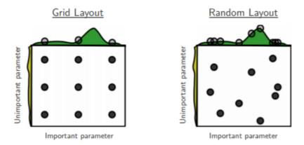
Figure 3.11: As shown in the figure, random search has found the optimal hyper-parameters less number of iterations. In grid search, however, the optimal hyper-parameter is not found since we do not have it in our grid.
