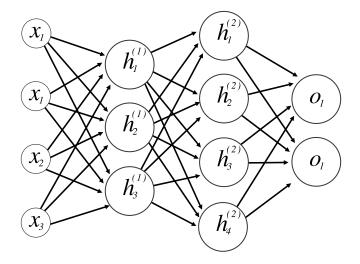
Figure 3.8: A simplified graphical visualization of the feed-forward neural network model. This FFNN takes 4 inputs, has 2 hidden layers  $h^{(1)}$  and  $h^{(2)}$  of sizes 3 and 4 respectively, and has an output layer of size 2. Biases were omitted only from this visualization. We can see how each two adjacent layers are fully connected to each other
