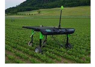
FIGURE 1.5: Autonomous mobile robot weeding a field [2]
