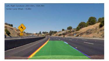
FIGURE 3.9: Tracing road by HSV method.
