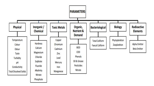
Figure 1.1: Water quality parameters.
