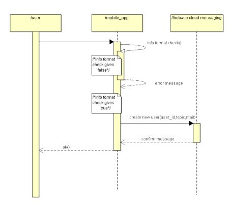
Figure 3.5: Registration Sequence Diagram
