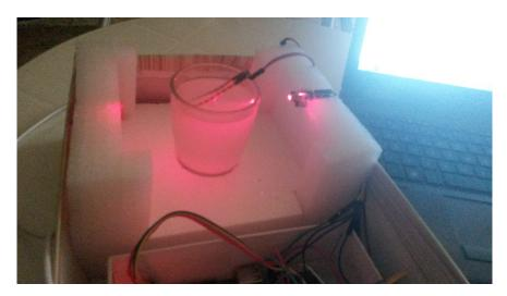
Figure 4.29: Very Turbid Water Check.
