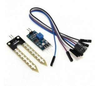
Figure 4.5: Soil Moisture Sensor(YL-69)
