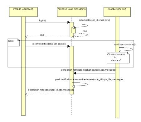
Figure 3.6: Notification Sequence Diagram
