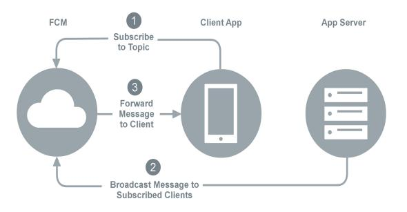
Figure 3.3: Notification With Firebase Cloud Messaging
