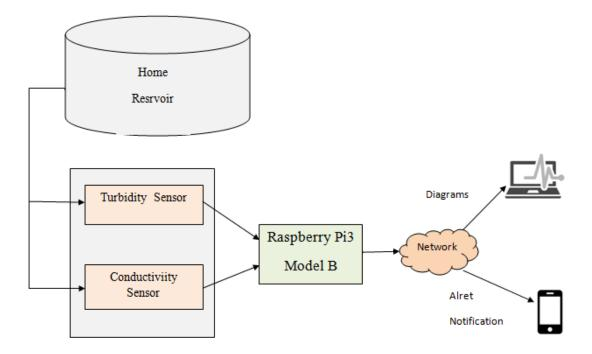
Figure 3.1: System Architecture of Our Proposed System.
