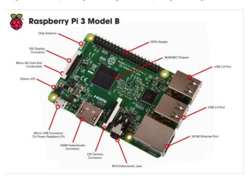
Figure 4.1: Raspberry Pi Model B.
