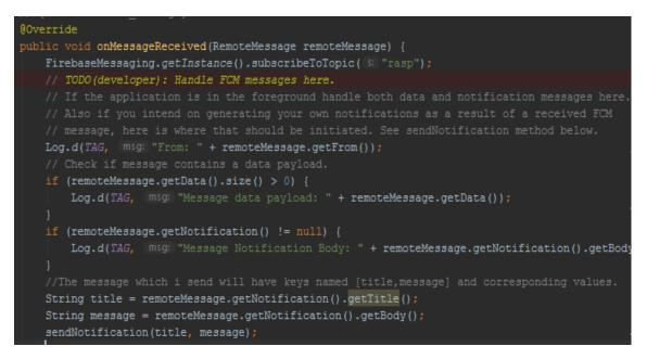
Figure 4.13: Receive Notification Source Code.
