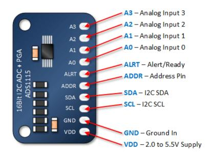
Figure 4.6: Analog To Digital Converter(ADS1115)
