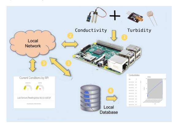
Figure 3.2: System Operations Diagram.
