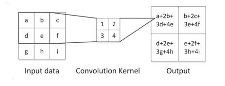
FIGURE 3.3: An example of convolution operation
