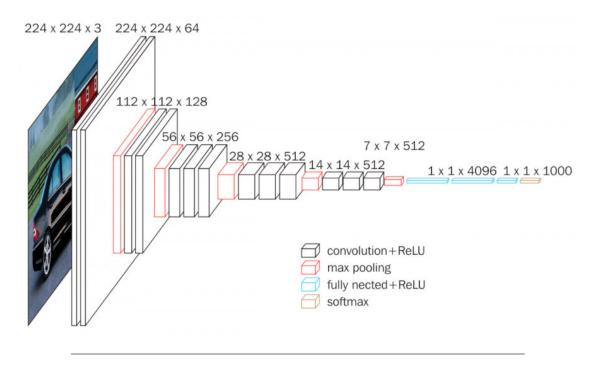
FIGURE 3.6: Base network VGG-16 architecture [19].
