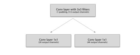
FIGURE 3.8: Convolutional implementation of an RPN architecture, where k is the number of anchors.
