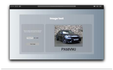
FIGURE 4.11: Extracting licence plate from an image.
