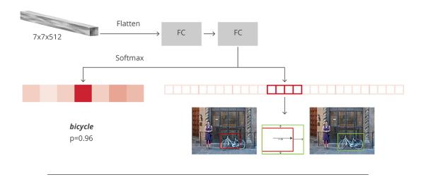
FIGURE 3.11: R-CNN architecture [21].
