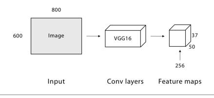
FIGURE 4.2: First step of FasterR-CNN.
