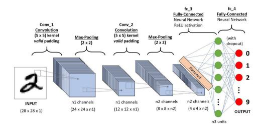
FIGURE 3.1: An example of CNN architecture
