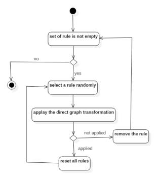
Figure 2.6: Non-deterministic Graph transformation activity diagram
