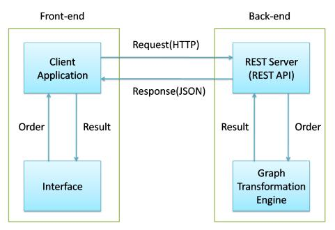
Figure 4.1: Graph transformation tools global architecture
