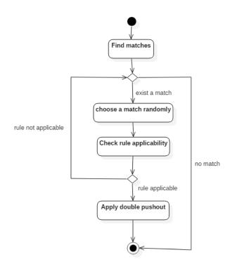
Figure 2.5: Direct graph transformation activity diagram
