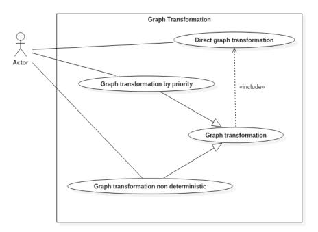
Figure 2.3: Graph transformation use case diagram
