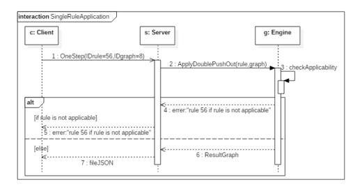
Figure 4.2: Sequence diagram of Single rule application
