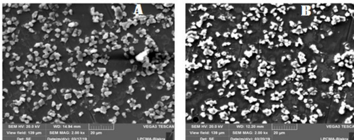
**Fig. III.9 SEM micrograph of the titania spin coating films with and without annealing: (A)  $\text{TiO}_2$  without annealing and (B) with annealing at 300 °C for 30 min**
