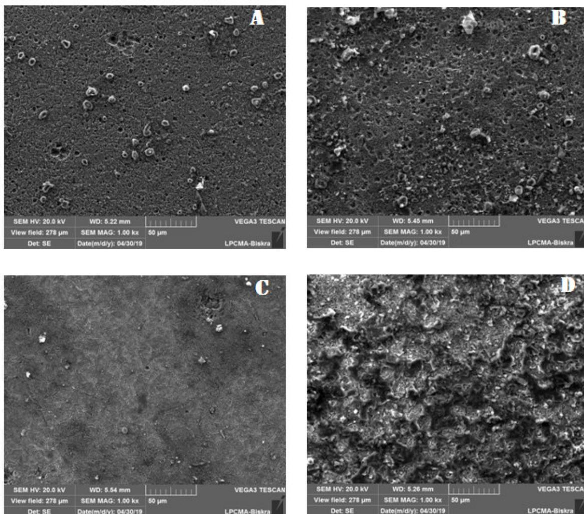
**Fig. IV.7. SEM images for Ti/TiO<sub>2</sub> multilayer coatings with (A) 2 layers, (B) 4 layers, (C) 6 layers and (D) 8 layers after corrosion test.**
