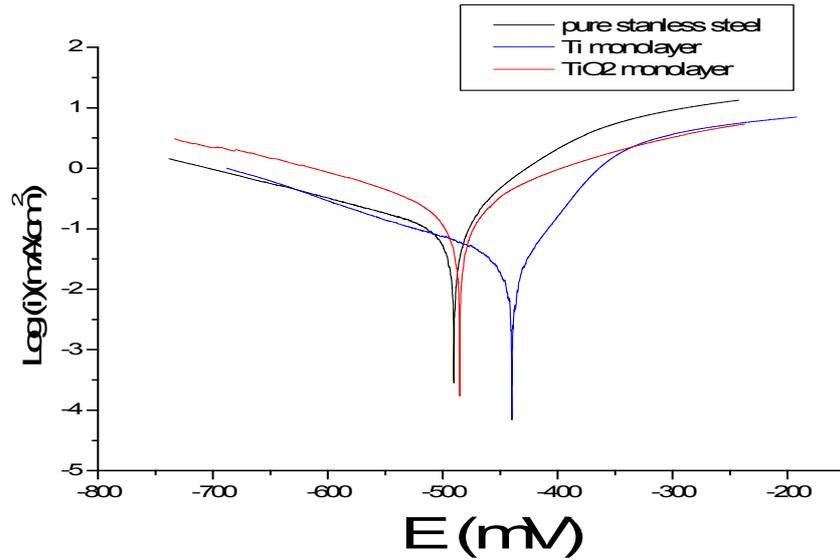
**Fig. IV.1 Potentiodynamic polarization behavior of stainless steel, Ti and TiO<sub>2</sub> monolayer in HCl solution**
