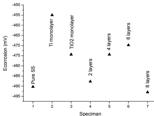
**Fig. IV.3. corrosion potential as function as the number of layers.**
