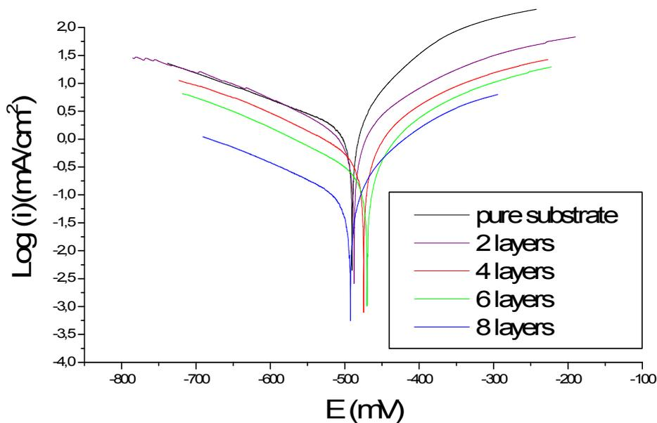
Fig. IV.2. Polarization curves of Ti/TiO<sub>2</sub> multilayer coatings with 2, 4, 6 and 8 films
