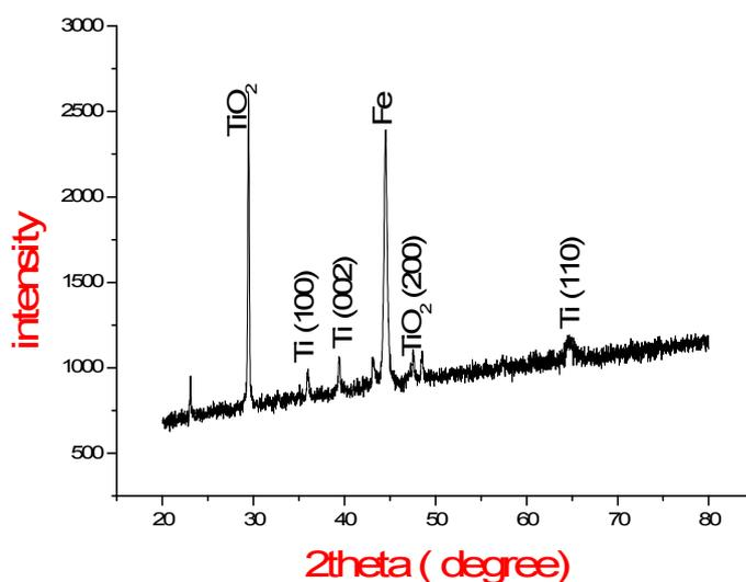
**Fig. III.4 XRD patterns of Ti electroplating thin films.**
