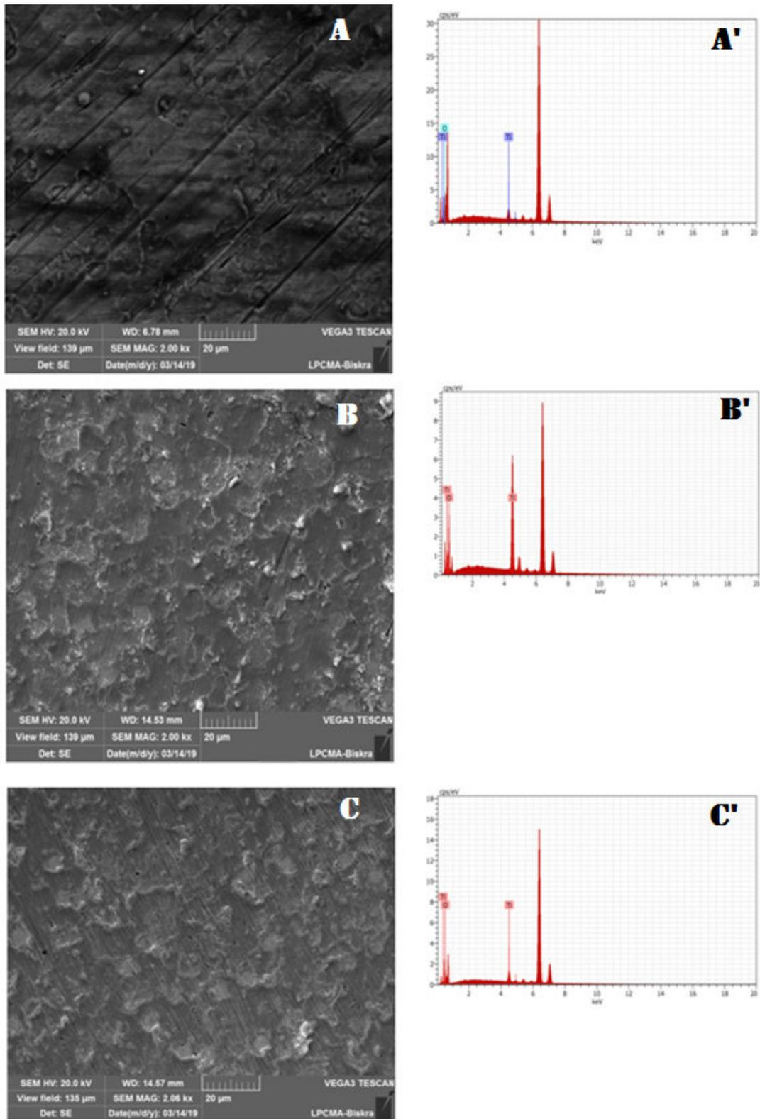
Fig. III.5. (A), (B) and (C)/(A'), (B') and (C') SEM/EDX image of TiO<sub>2</sub> thin films deposit in 4000 rpm for 30, 45 and 60 seconds on stainless steel substrate using spin coater method respectively
