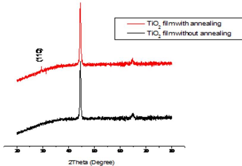
**Fig. III.8. X-ray Diffractogrammes of  $\text{TiO}_2$  monolayer deposited on stainless steel with and without annealing**
