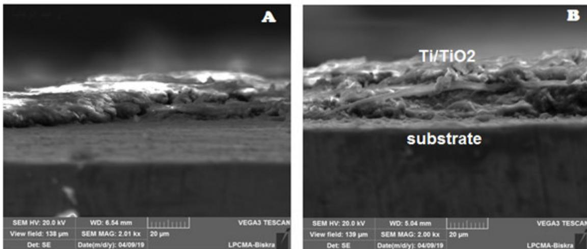
**Fig. III.14 Cross-section SEM images for Ti/TiO<sub>2</sub> multilayer with 4 and 6 films (A):4 layers and (B):6 layers**
