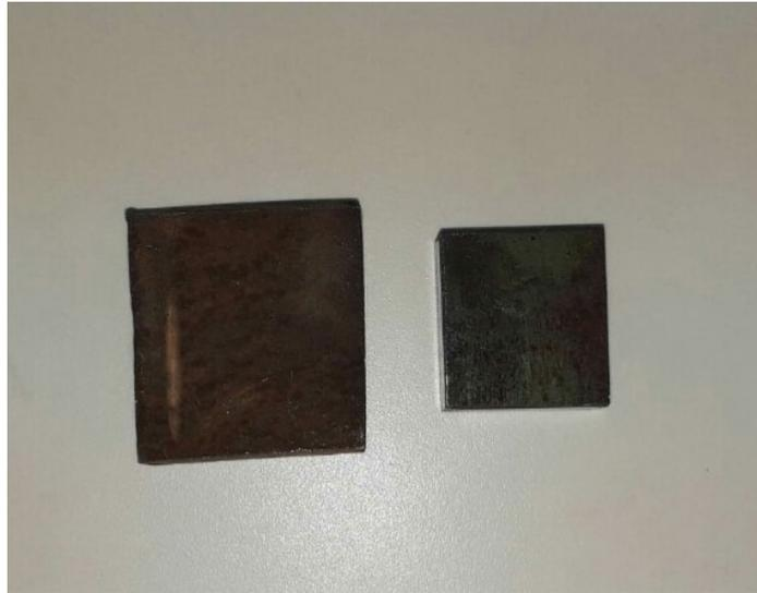
**Fig. II.1** Stainless steel X70 after cutting
