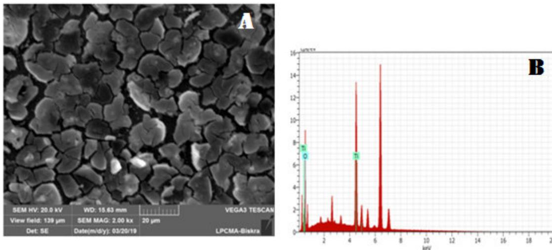
**Fig.III.12. SEM/EDX images for Ti/TiO<sub>2</sub> multilayer with 6 films deposited on stainless steel.**
