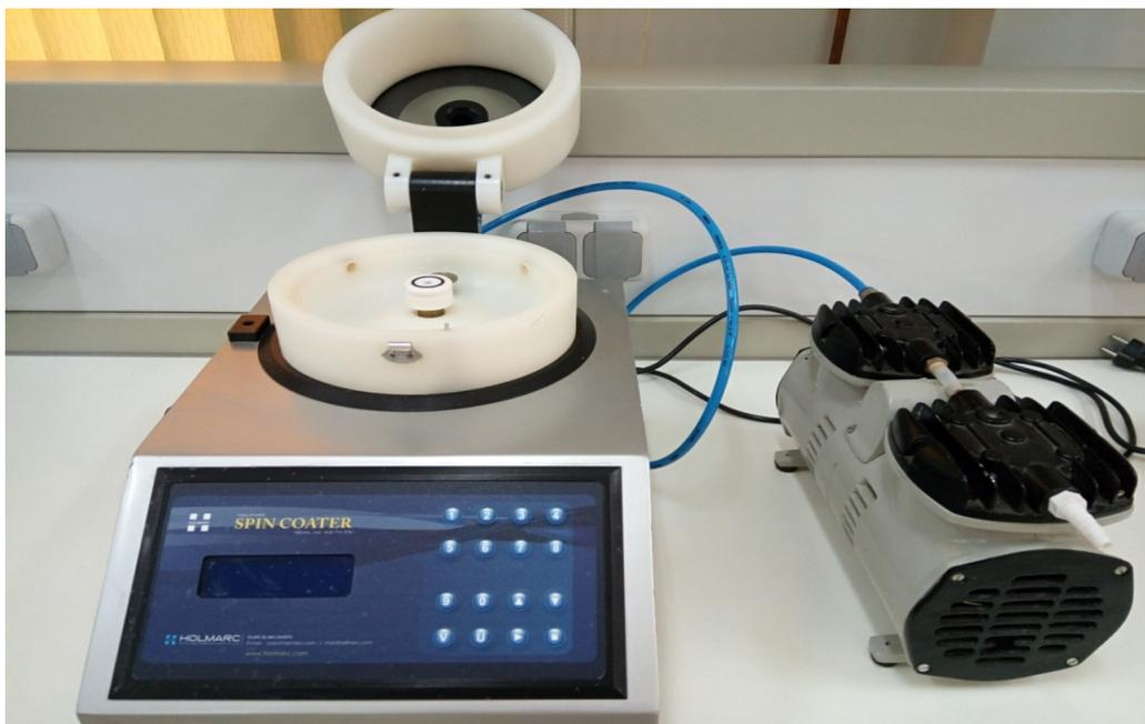
**Fig. II.4 Spin coater HOLMARC device**
