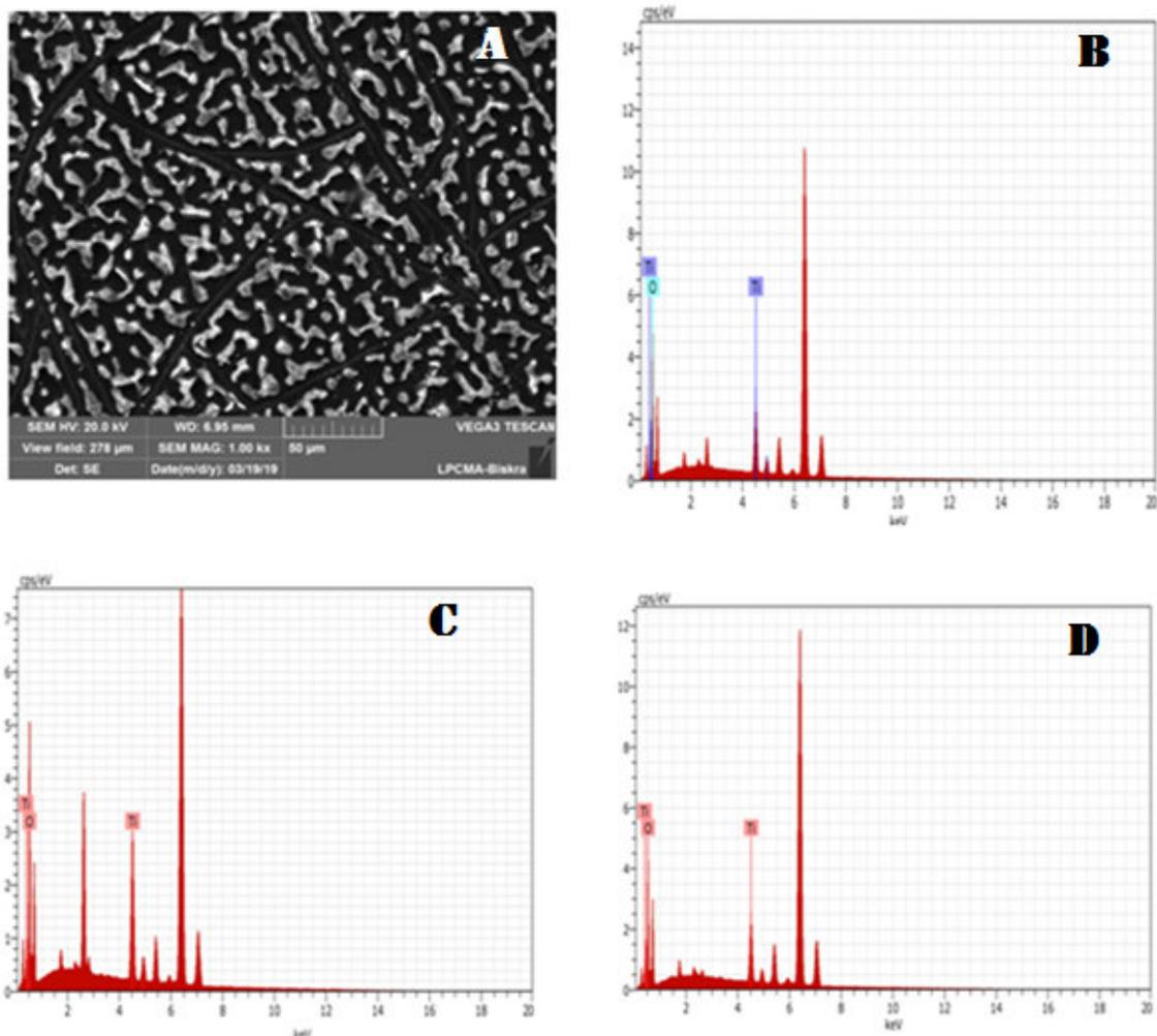
**Fig. III.10 SEM/EDX images for Ti/TiO<sub>2</sub> multilayer with 2 films: (A): SEM image of the Ti/TiO<sub>2</sub> multilayer with 2 films, (B) EDX spectrometer of the black region, (C) EDX spectrometer of the white region, (D)EDX spectrometer of the grey region**
