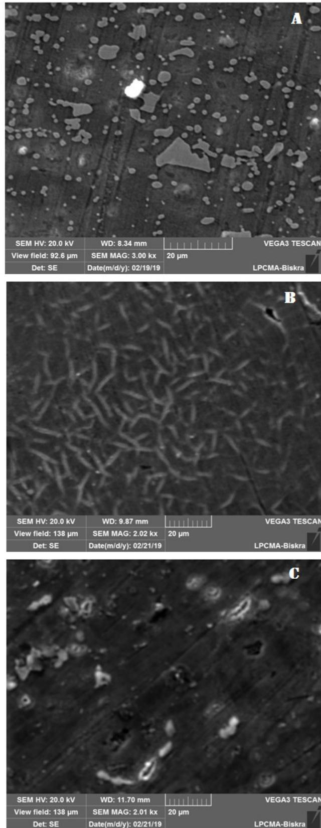
Fig. III.3 SEM images of Ti electroplating deposited under (A) room temperature, (B) 30 °C and (C) 50 °C.
