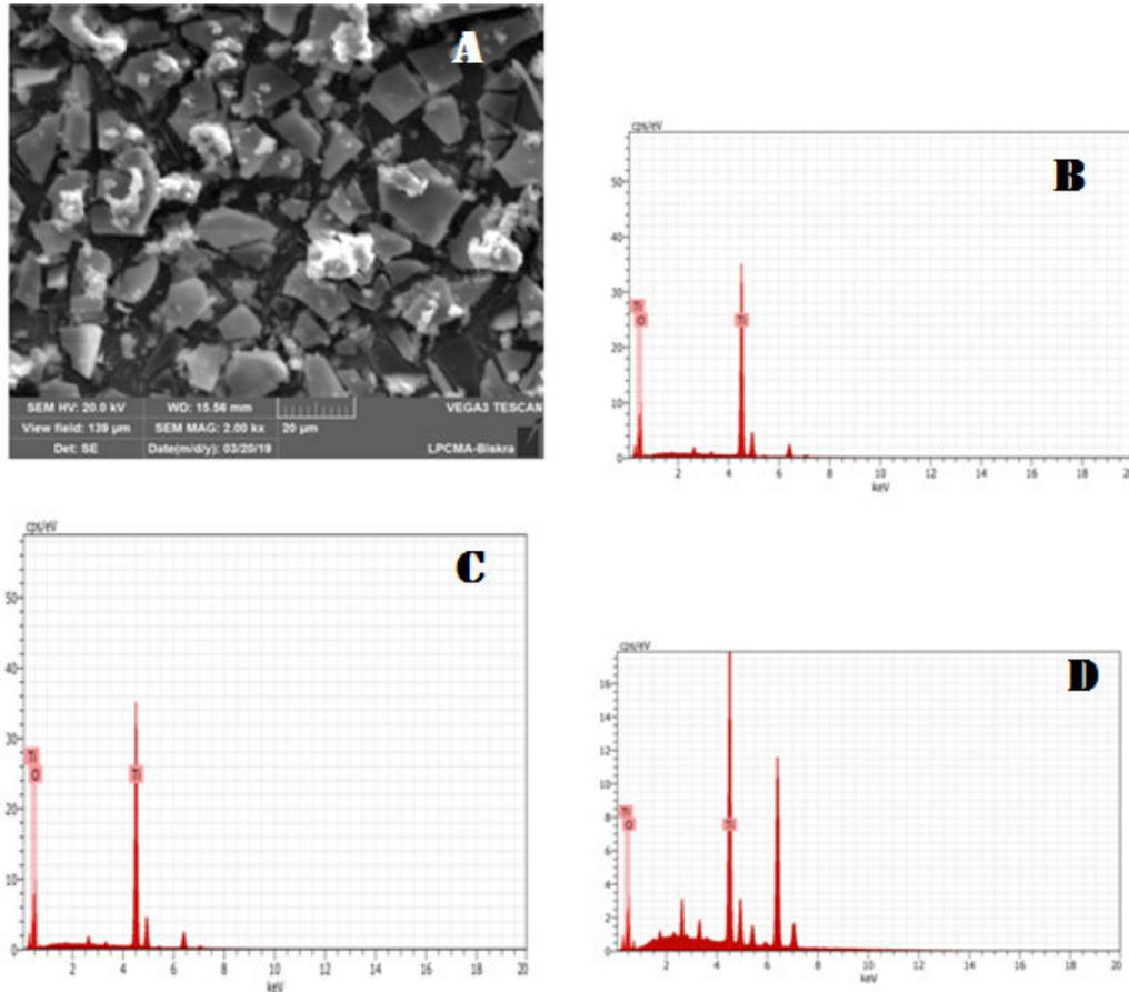
**Fig.III.11: SEM/EDX images of Ti/TiO<sub>2</sub> multilayer with 4 films deposited on stainless steel: (A) SEM image of the Ti/TiO<sub>2</sub> multilayer with 4 films, (B) EDX spectrometer of the grey region, (C) EDX spectrometer of the global surface and (D) EDX spectrometer of the black region.**
