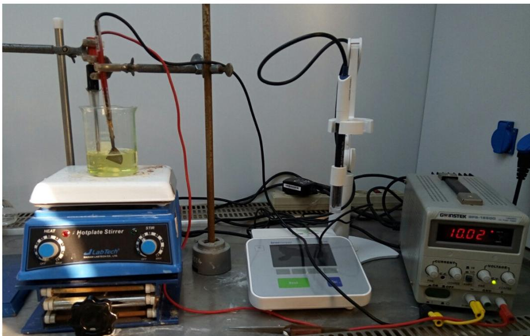
**Fig. II.3 The Electrodeposition process**
