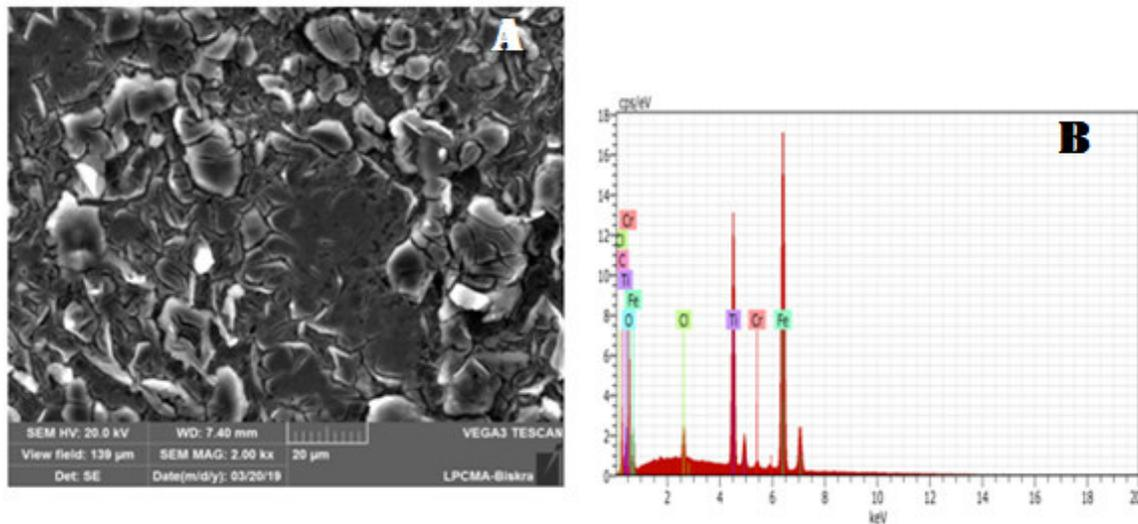
**Fig. III.13 SEM/EDX images for Ti/TiO<sub>2</sub> multilayer with 8 films deposited on stainless steel.**
