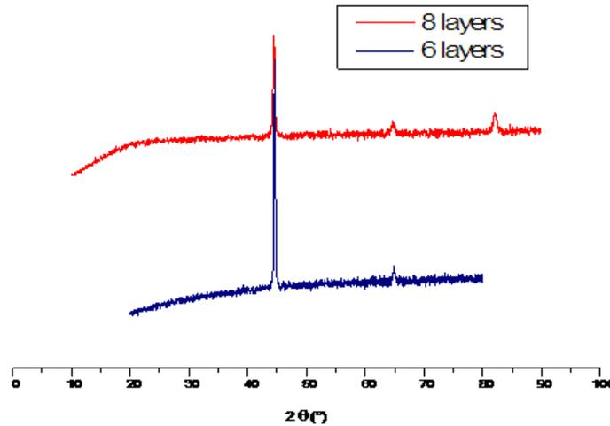
**Fig.III.15. X ray Diffractogrammes of Ti/TiO<sub>2</sub> multilayer coatings with 6 and 8 layers.**
