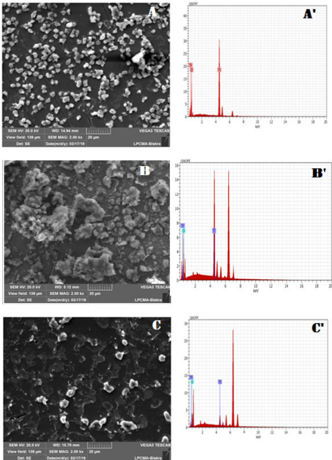
Fig. III.7 (A), (B) and (C)/(A'), (B') and (C') SEM/EDX image of  $\text{TiO}_2$  thin film deposit with 0.5, 0.6 and 0.8 mol/L at 5000 rpm for 45 seconds on stainless steel substrate using spin coater method respectively.
