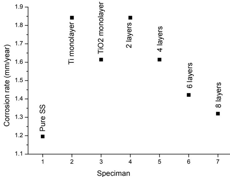
**Fig. IV.5 Corrosion rate in terms of nature of specimens**
