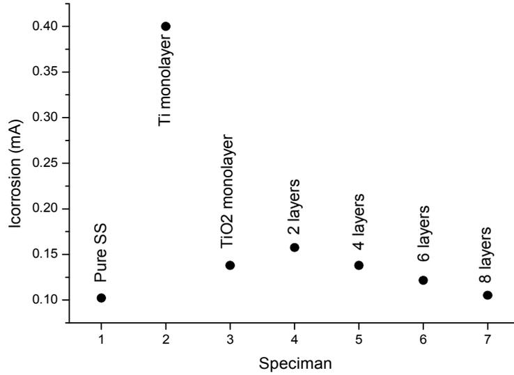
**Fig.IV.4. Corrosion current density in terms of number of layers**
