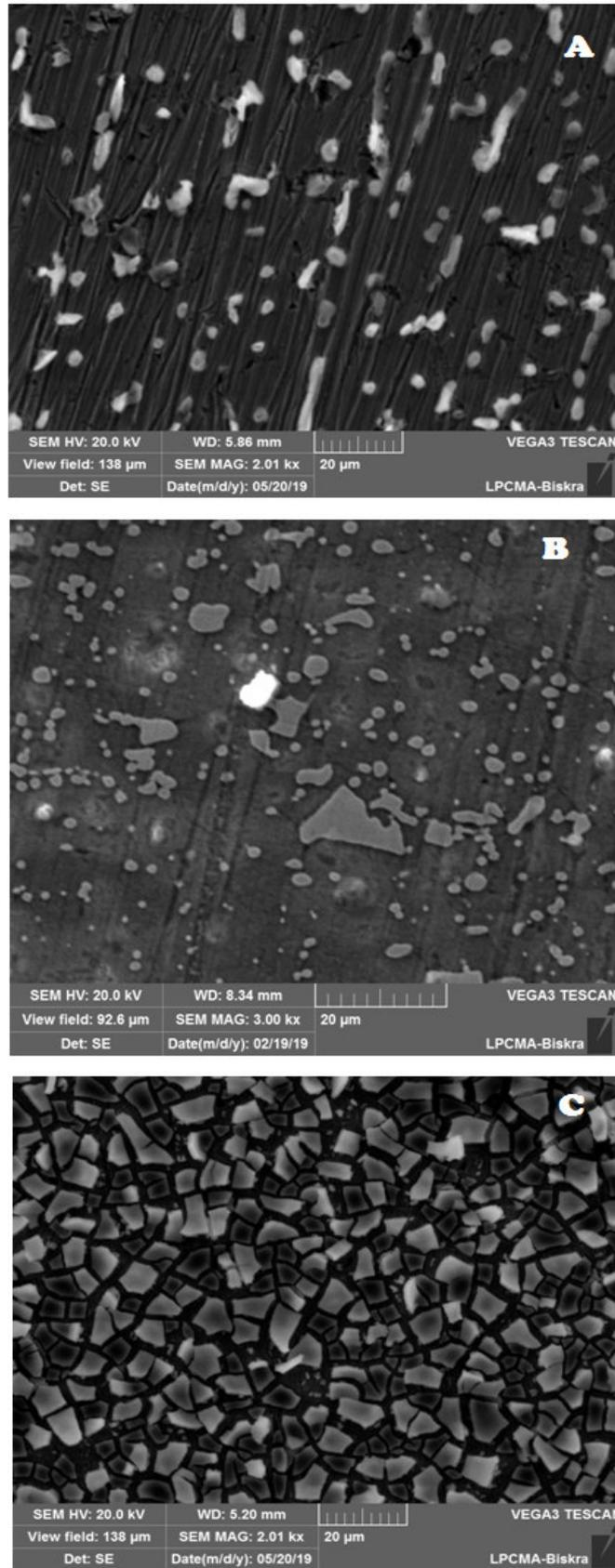
Fig. III.2 SEM results of Ti thin film deposited at 15 V for 4 min (A), 5 min (B) and 8 min (C) respectively.
