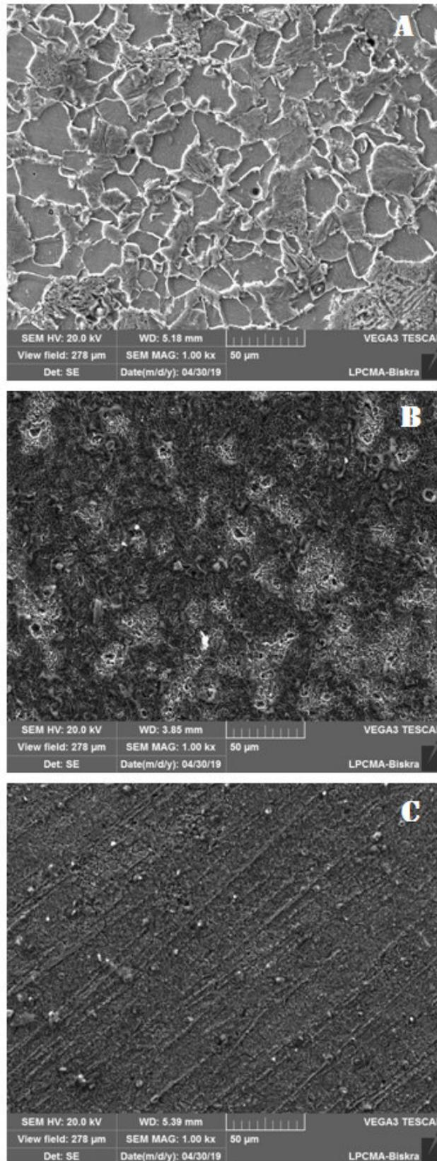
Fig. IV.6. SEM characterization of Ti, TiO<sub>2</sub> monolayer and stainless steel after corrosion test in 10 wt% HCl solution
