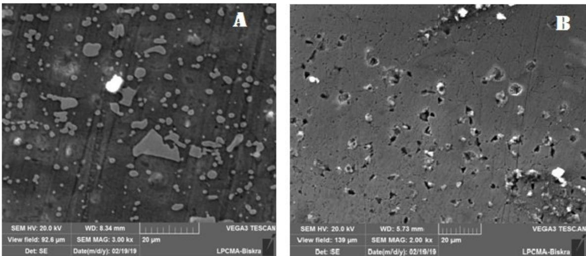
**Fig. III.1. SEM images for Ti thin film applied by (A) 15 V and (B) 18 V.**
