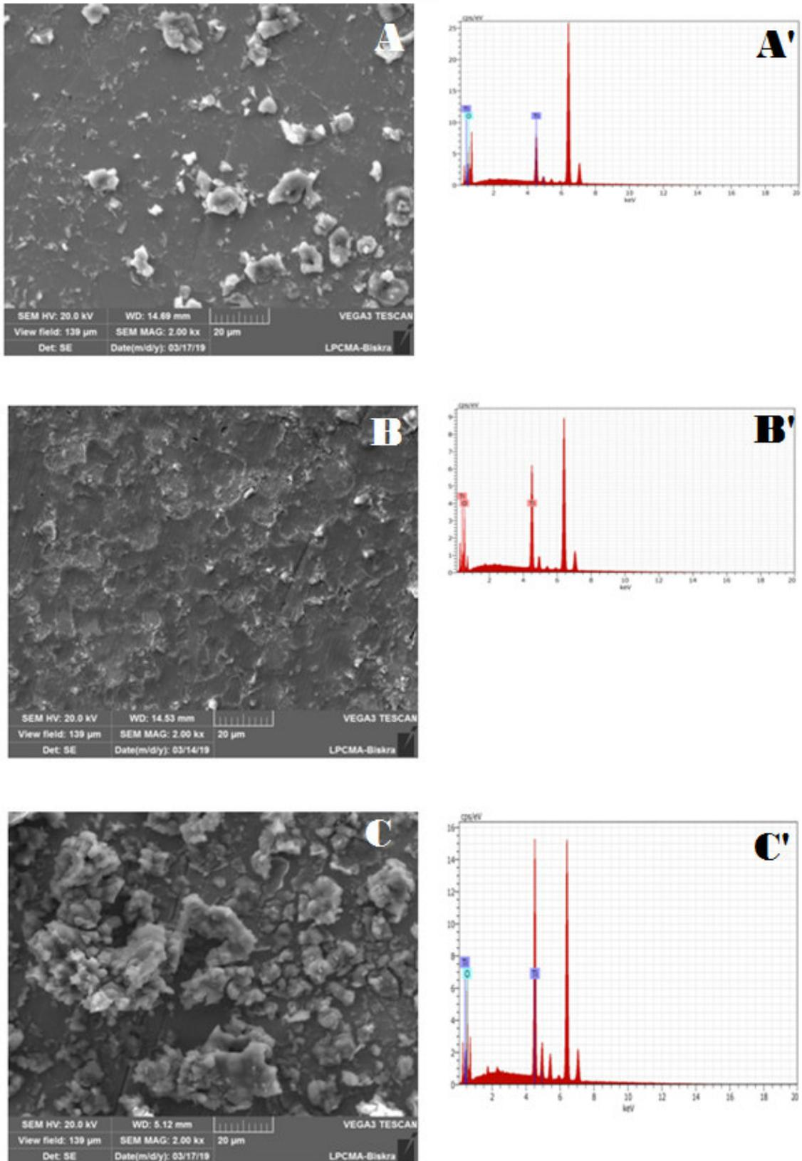
Fig. III.6 (A), (B) and (C)/(A'), (B') and (C') SEM/EDX image of TiO<sub>2</sub> thin film deposit in 2000, 4000 and 5000 rpm for 45 seconds on stainless steel substrate using spin coater method respectively
