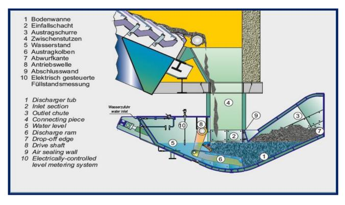
Figure 38: discharge invention. Source: [MAR 13]
