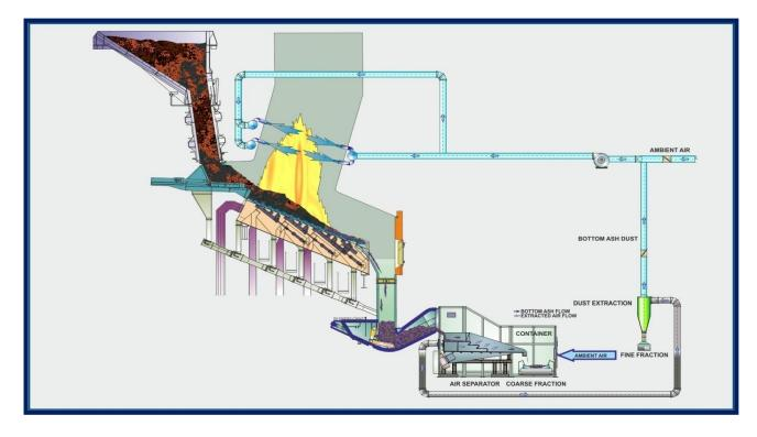
Figure 42: Dry discharge system. Source: [MAR 13]
