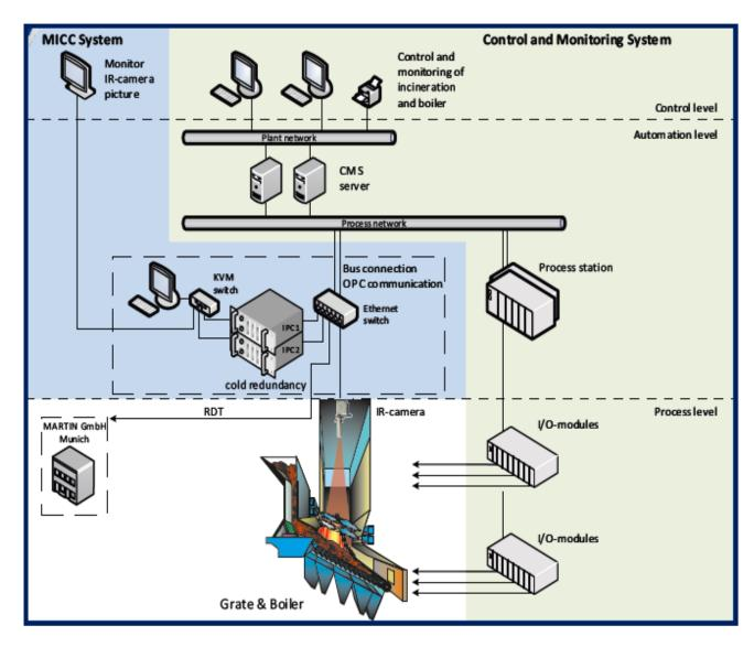
Figure 41: MICC - MARTIN Infrared Combustion Control. Source: [MAR 13]
