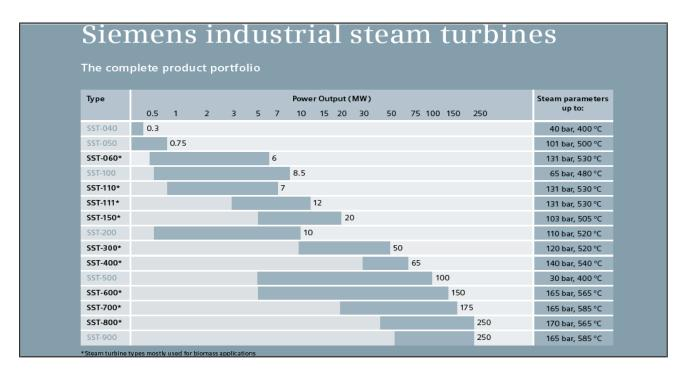
Figure 20: Siemens industrial steam turbines. Source: [SIE 17]
