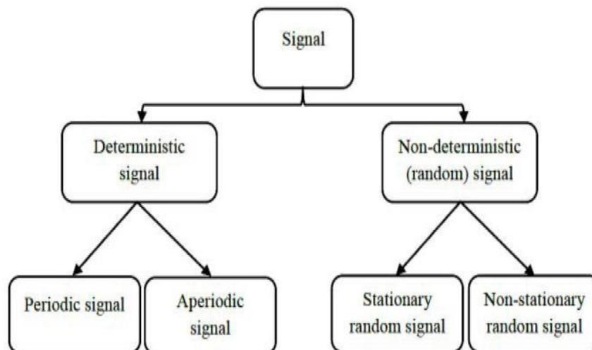
**Figure.II.1.** Schematic diagram of signal classification [17].
