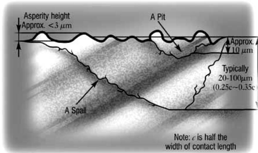
**Figure III.12** Pitting and spalling [7].
