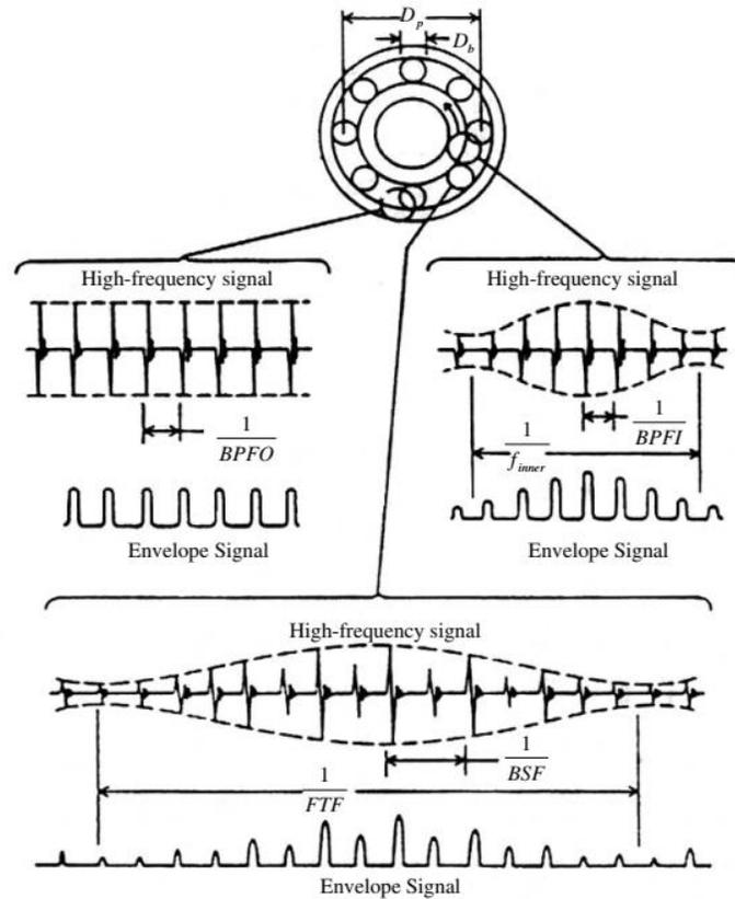
**Figure III.9** Typical vibration signals generated by local faults in rolling element bearings (stationary outer race) BPFO, BPFI [6].
