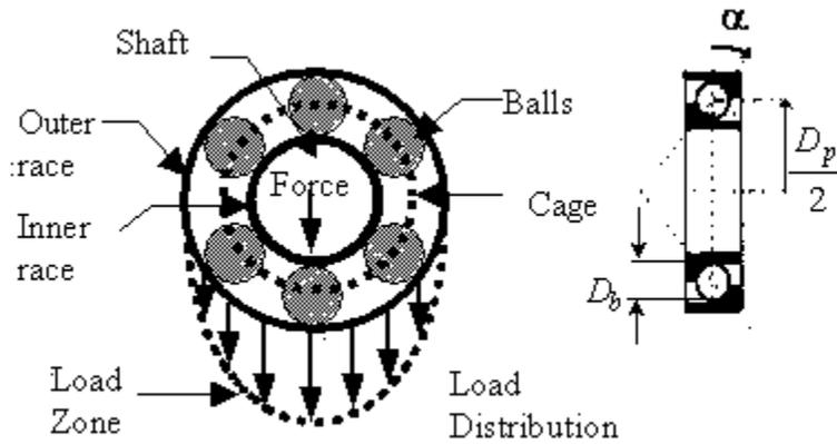
**Figure III.3.** Rolling bearing components and load distribution for a fixed outer race [6]
