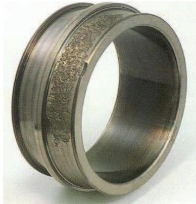
**Figure III.11.** Ripple pattern flaking of a tapered roller bearing [14].
