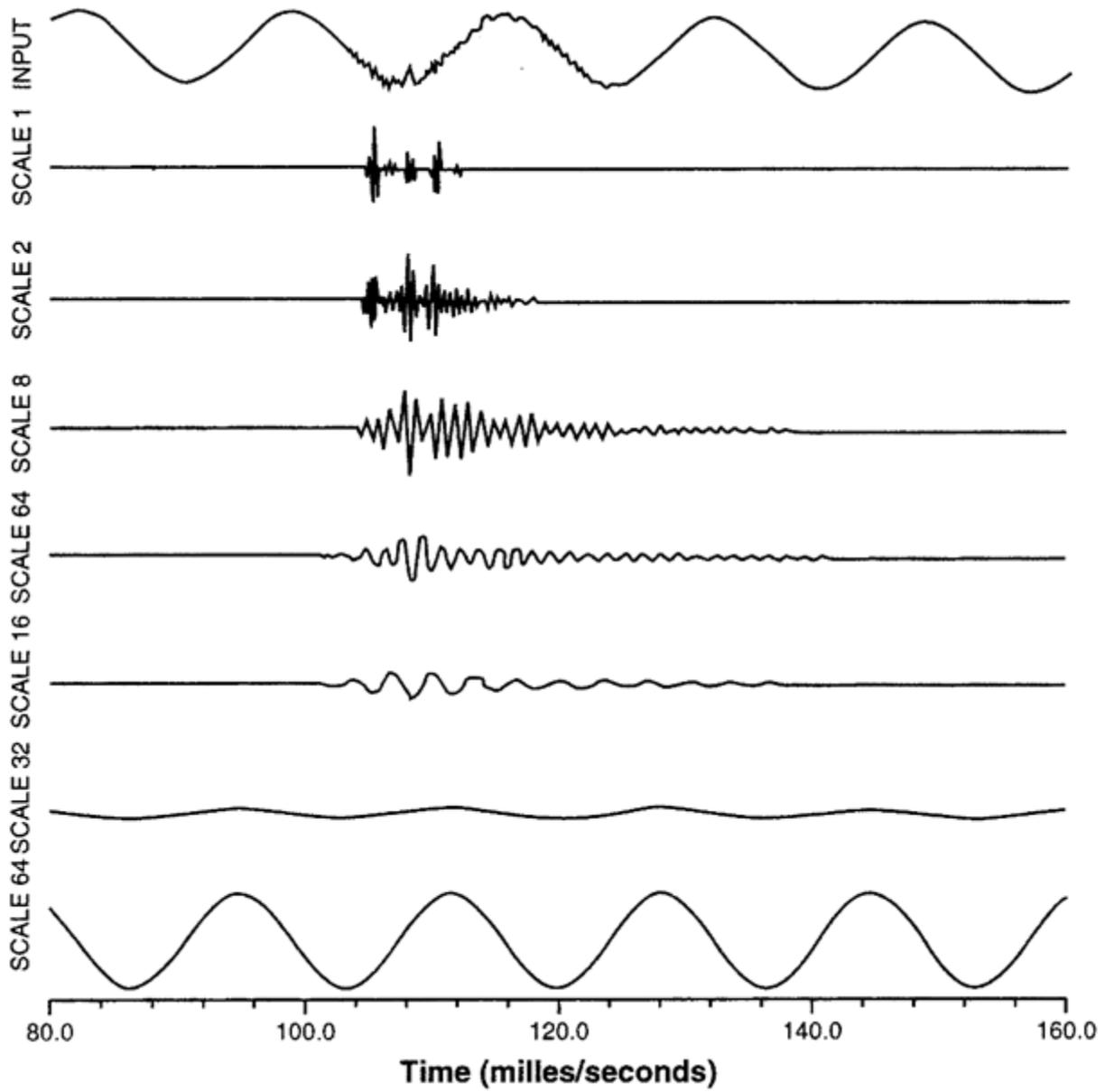
**Figure.II.7.** Multiresolution wavelet analysis of a transient signal [6].
