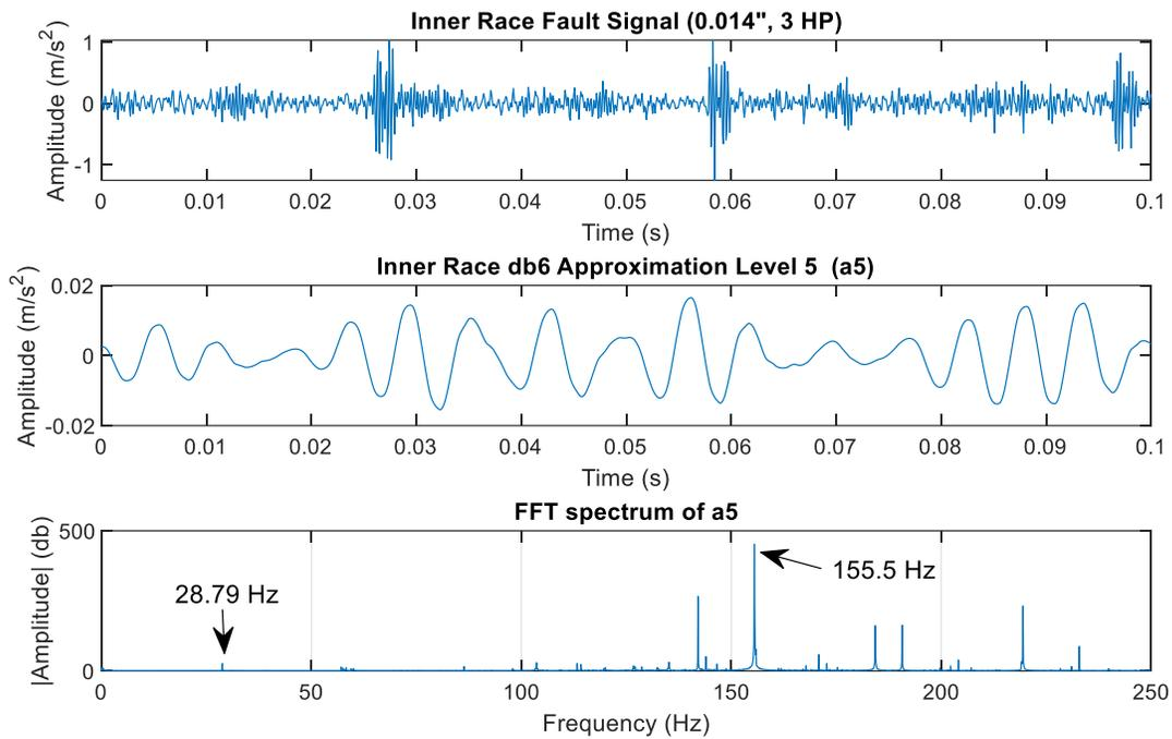
**Figure.IV.10.** The 3 levels of the applied method for inner race fault signal (3HP, 0.014")
