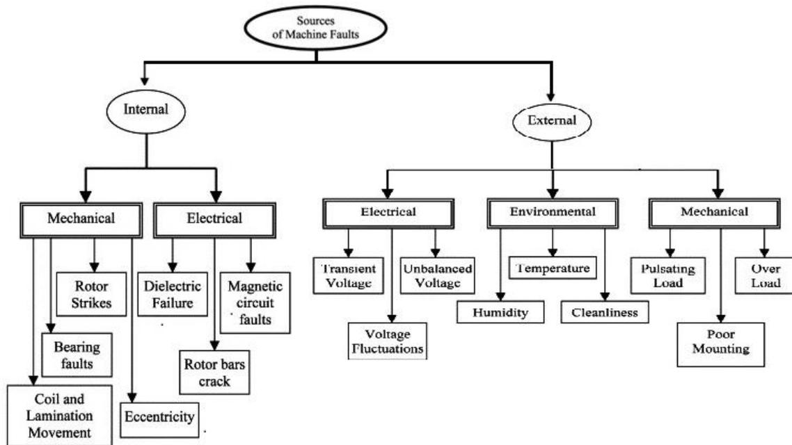
**Figure I.5.** Different failures modes [4].
