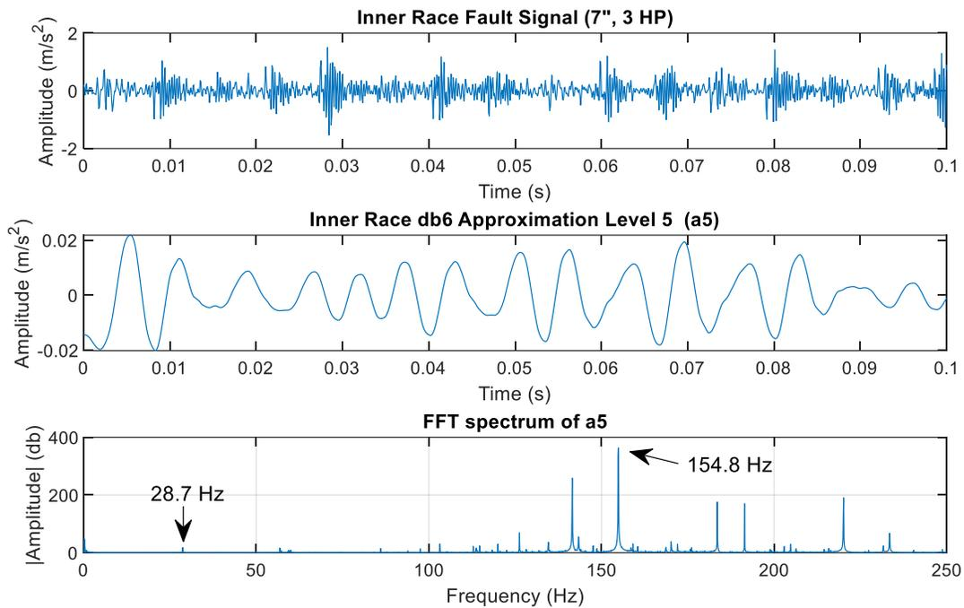
**Figure.IV.8.** The 3 levels of the applied method for inner race fault signal (3HP, 0.007")
