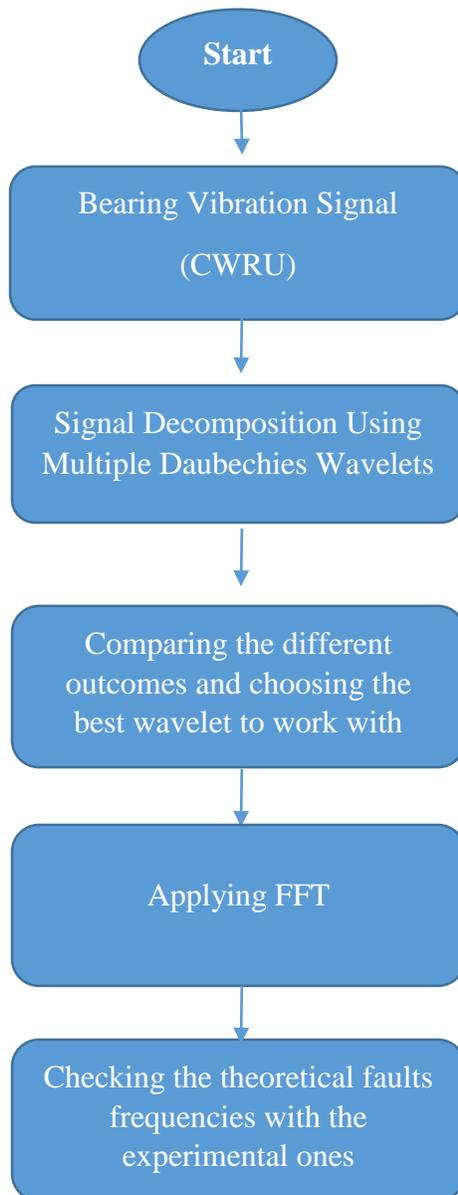
**Figure IV.2.** Flowchart of the proposed work methodology
