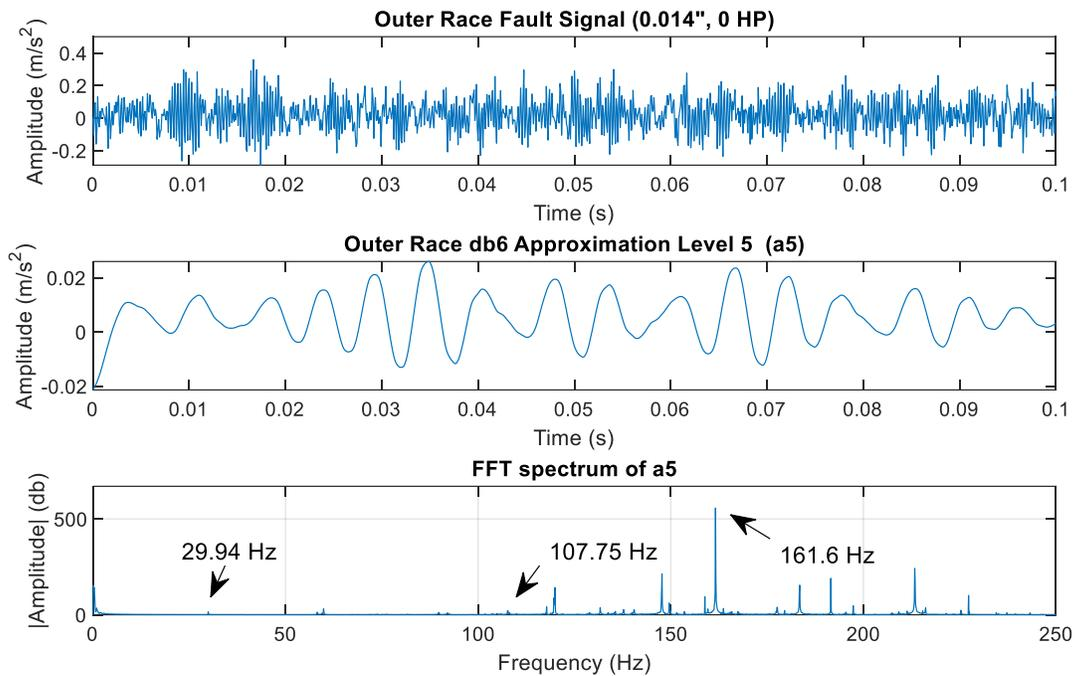
**Figure.IV.13.** The 3 levels of the applied method for outer race fault signal (0HP, 0.014")
