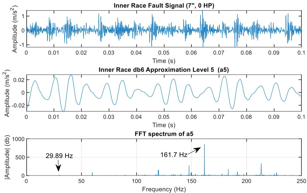
**Figure.IV.7.** The 3 levels of the applied method for inner race fault signal (0HP, 0.007")
