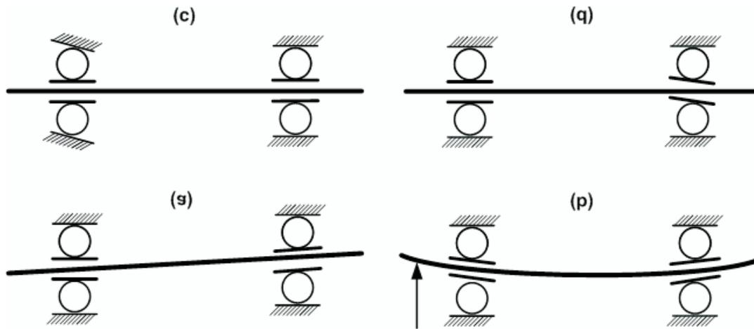
**Figure III.7.** (a) Misalignment (out-of-line), (b) shaft deflection, (c) crooked or tilted outer race, (d) crooked or tilted inner race [11].
