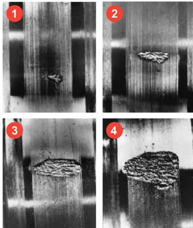
**Figure III.4.** Evolution of a bearing defect [9].
