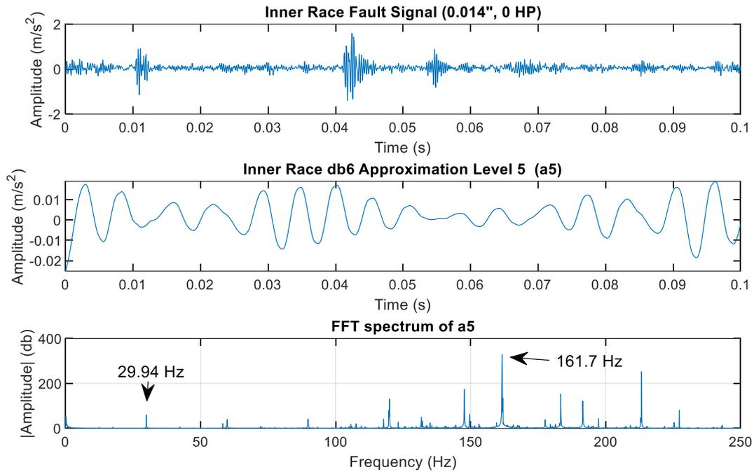
**Figure.IV.9.** The 3 levels of the applied method for inner race fault signal (0HP, 0.014")
