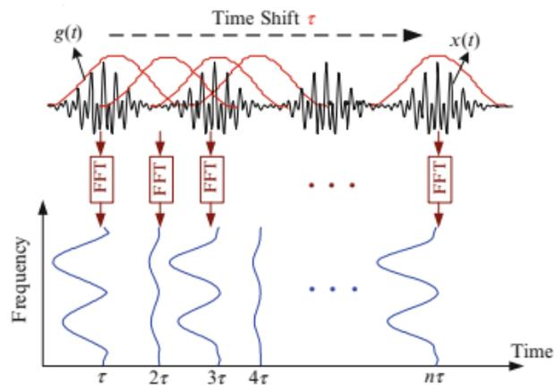
**Figure II.3.** Illustration of short-time Fourier transform on signal  $x(t)$  [18].
