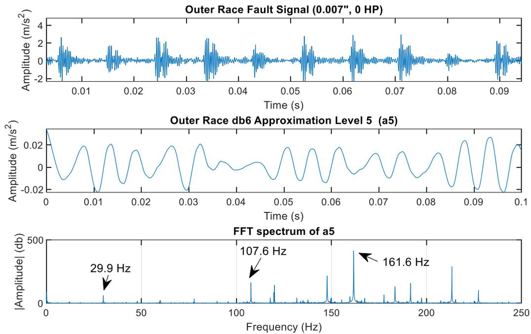
**Figure.IV.11.** The 3 levels of the applied method for outer race fault signal (0HP, 0.007")
