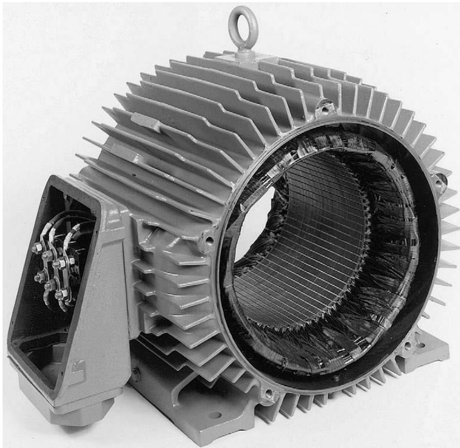
**Figure I.2.** Stator of three-phase induction motor [3].
