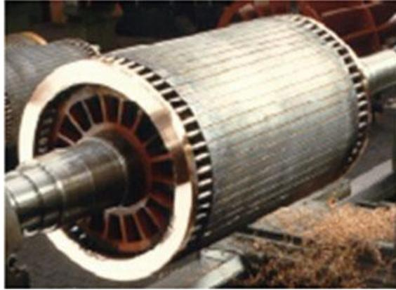
**Figure I.3.** Squirrel-cage rotor [1]
