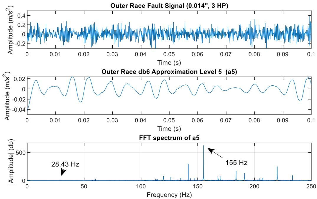
**Figure.IV.14.** The 3 levels of the applied method for outer race fault signal (3HP, 0.014")
