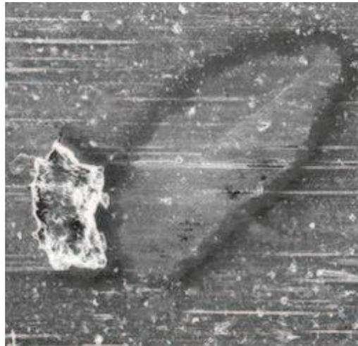
**Figure III.6.** Inner raceway spall originating on the surface from previous damage in the form of an indentation [14].
