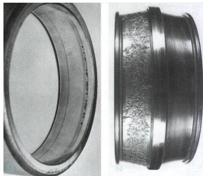
**Figure III.8.** Bearing in advanced state of deterioration [9].
