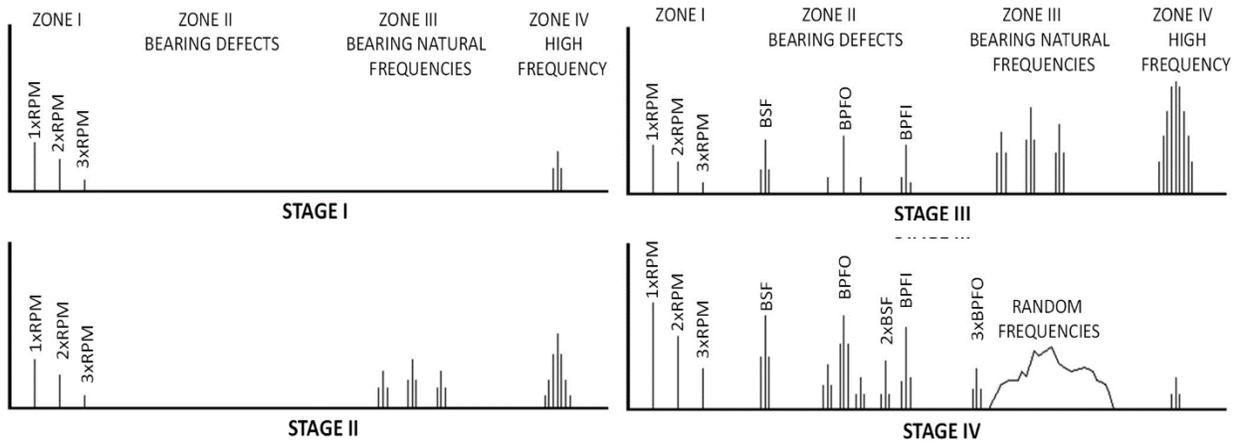
**Figure III.10.** Bearing damage stages [15].
