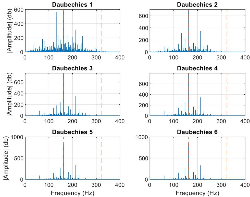
**Figure.IV.4.** Inner race fault sample.
