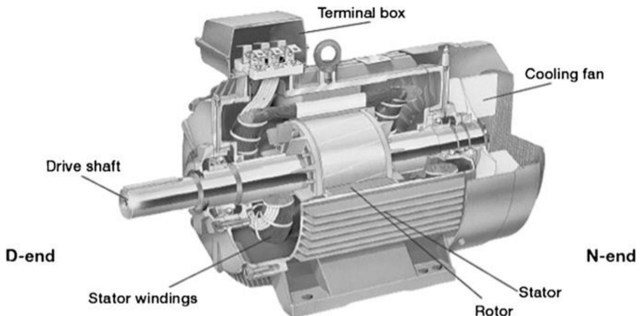
**Figure I.1.** AC Induction Motor(dissected) [1]
