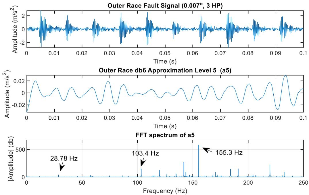
**Figure.IV.12.** The 3 levels of the applied method for outer race fault signal (3HP, 0.007")
