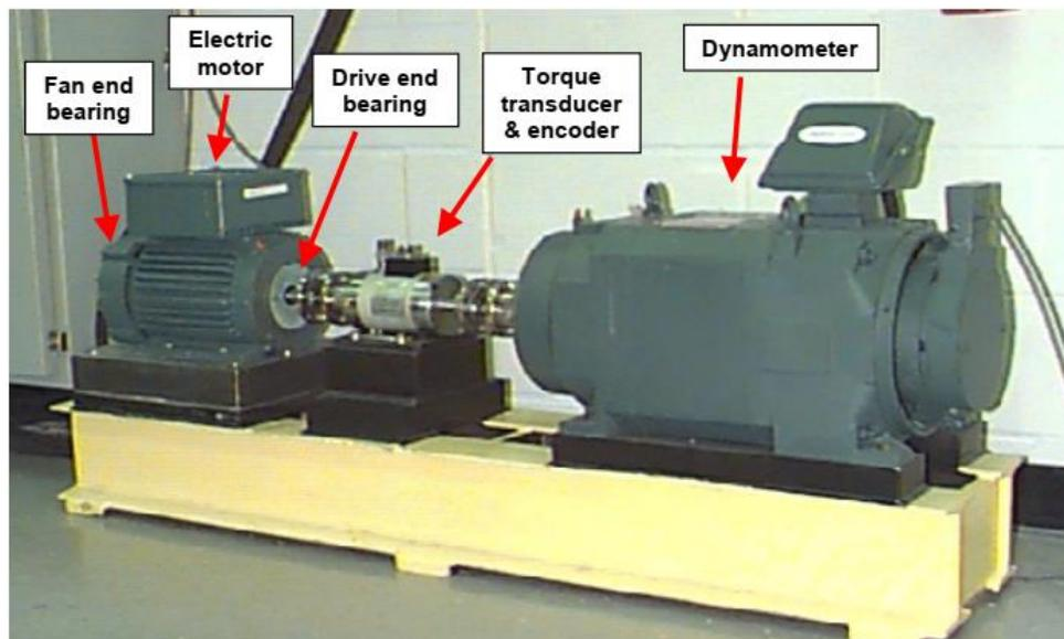
**Figure.IV.1.** Bearing test stand used by Case Western Reserve University (CWRU) [19].
