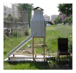
Fig (II-23): Photo of the tested solar dryer.
