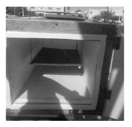
Fig (III-6): Support of the drying product.
