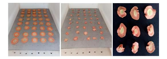
Fig (III-13): Wet and dried slices of carrot with 1mm of thickness and 30mm of diameter.
