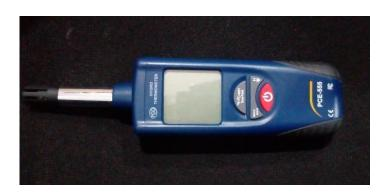
Fig (III-12): Hygrometer (Model PCE-555).
