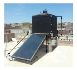
Fig (II-36): The experimental solar dryer.
