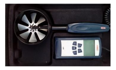
Fig (III-14): A digital anemometer (Model KIMO-LVA).
