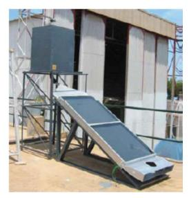
Fig (I-11): The indirect solar dryer [19].
