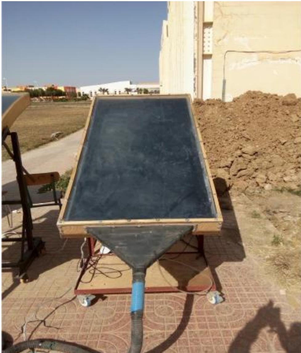
**Figure II.1:** The tested flat plate collector.
