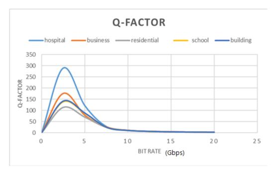
Figure 3.35: Variation of the Q-factor according to the bit rate
