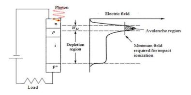
*Figure 1.5*: Avalanche photodiode showing high electric field region [7]
