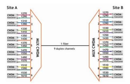
Figure 2.25: Transmission CWDM mux/demux [33]
