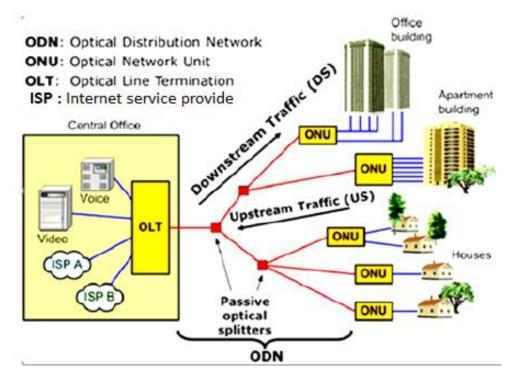
Figure 2.7: Passive Optical Network architecture [22]
