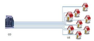
Figure 2.5: Point to point access topology [19]
