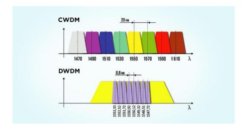
Figure 2.24: Wavelengths bands CWDM and DWDM [34]
