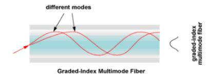
*Figure 1.11*: *Graded-Index Multimode fiber* [10]
