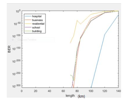
Figure 3.33: Variation of the BER according to the length of the fiber
