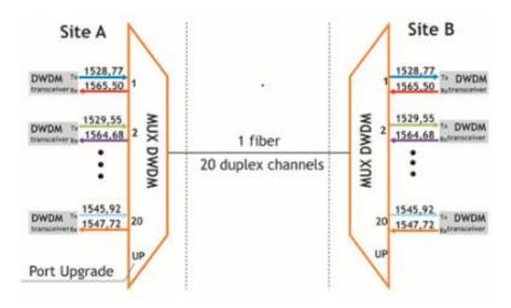
Figure 2.26: Transmission DWDM mux/demux [33]
