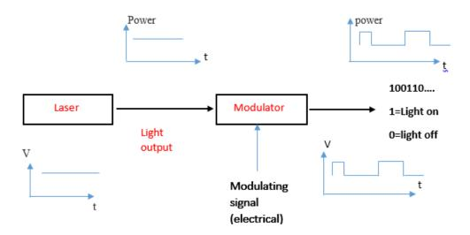
Figure 1.3: Laser diode used as optical external modulation
