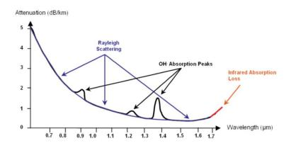
Figure 1.12: Typical Attenuation vs. Wavelength [14]
