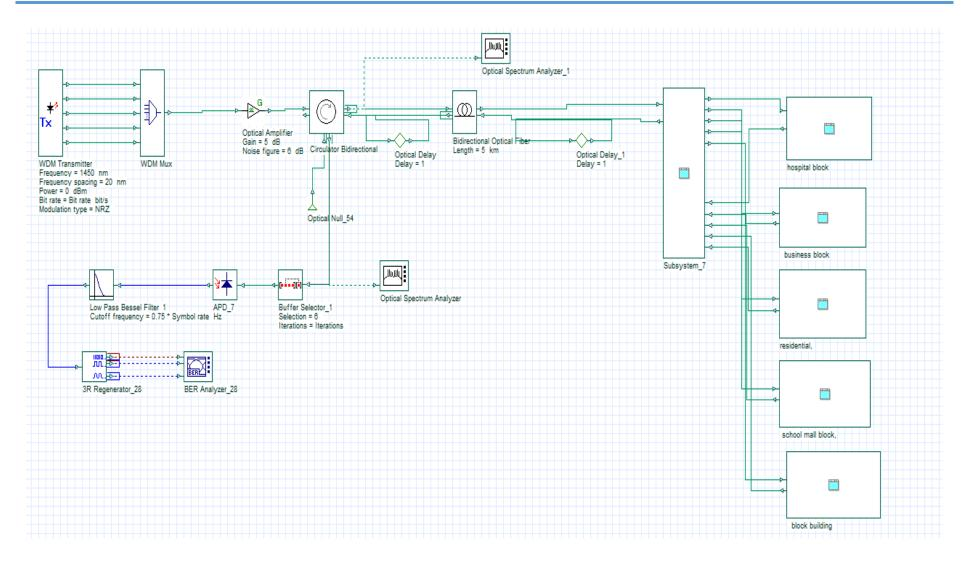
Figure 3.10: WDM GPON – Complete design
