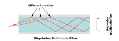
Figure 1.10: Step-Index Multimode fiber [10]
