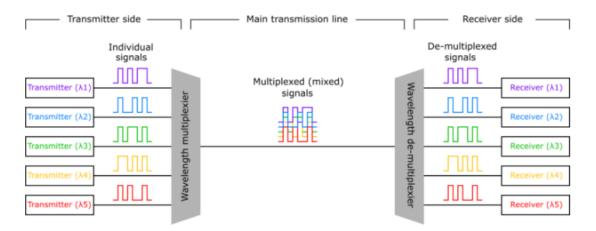
Figure 2.22: Schematic of WDM transmission system [32]
