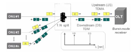
Figure 2.15: PON architecture based on time division multiplexing (TDM) [25]
