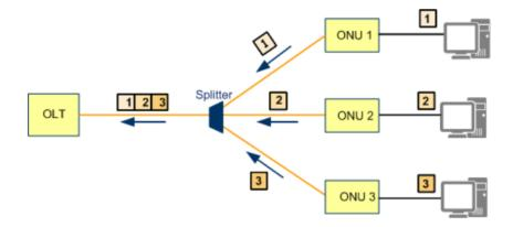
Figure 2.20: GPON TDMA to Upstream [29]
