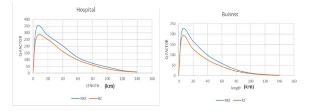
Figure 3.39: Comparison of the Q-factor RZ / NRZ as a function of distance
