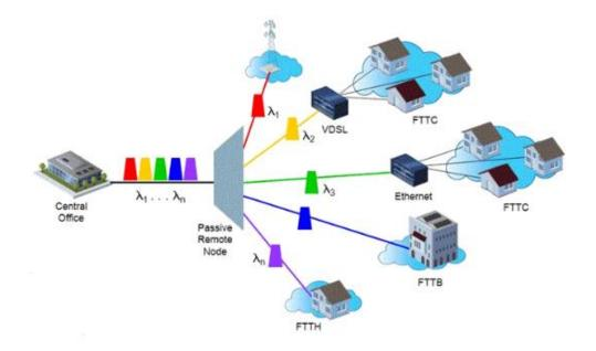
*Figure 2.23*: PON based on wavelength division multiplexing (WDM) [33]
