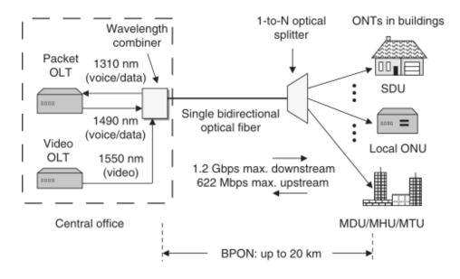
Figure 2.17: Basic BPON architecture and operational concept [18]
