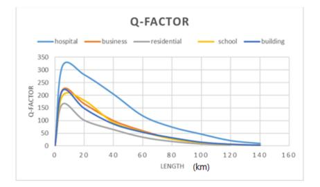
Figure 3.34: Variation of the Q-factor according to the length of the fiber
