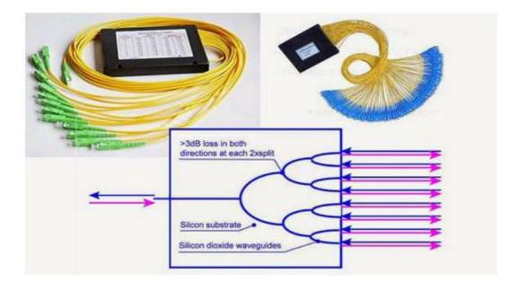
Figure 2.11: Schematic drawing for PLC Splitter [20]
