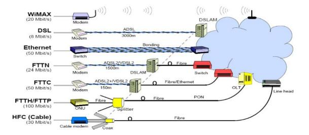
Figure 2.1: Access Network (Air, Copper, and Fibre access) [16]
