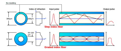
Figure 1.9: Multimode optical fibers (MMF) [4]
