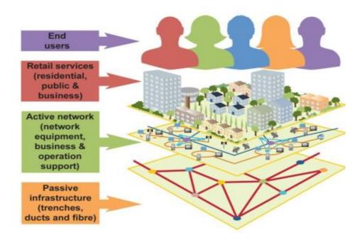
Figure 3.3: FTTx Network layers [41]
