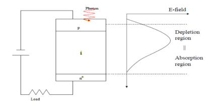
*Figure 1.4*: PIN photodiode showing combined absorption and depletion [7]
