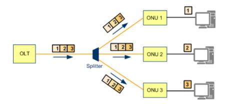
Figure 2.19: GPON Broadcasting to Downstream [29]
