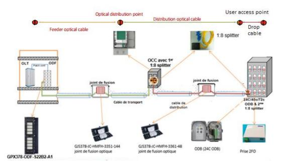
Figure 2.9 : Optical Distribution Network (ODN)
