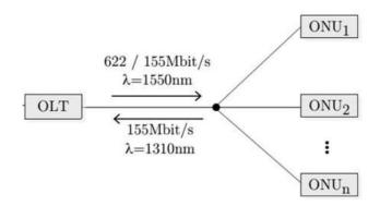
Figure 2.16: Typical APON network according to ITU-T G.983 [20]
