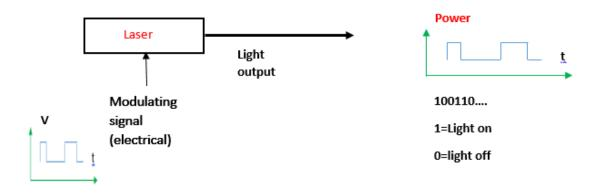
Figure 1.2: Laser diode used as optical direct modulation
