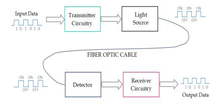
*Figure 1.1:* Basic fiber optical communication system [1]
