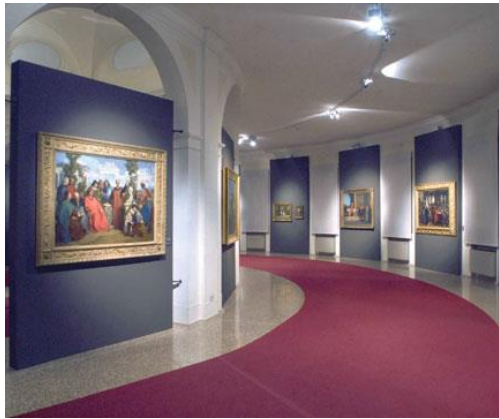
Figure 104. The directional light of spot lamps raises the brightness for exhibits – here with an appropriate beam angle for paintings.
