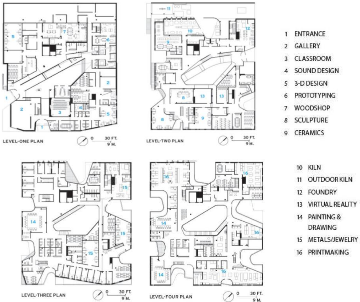
Figure 114 the project's plans source: stenholl architect
