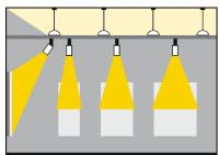
Fig (I-16) Indirect and direct components produce diffuse and directional lighting respectively Source: (Licht, 2018)
