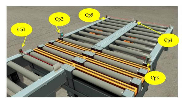
Figure III7: Position of the sensors in the Chain Transfer.
