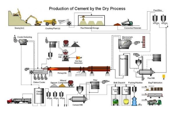
Figure I.1: Cement manufacturing cycle.
