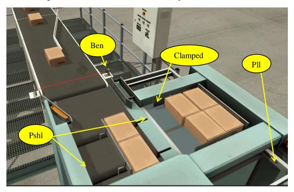
Figure III.4: Position of the sensors in the palletizer at the top.
