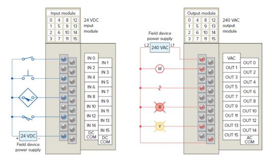
Figure II.5: Typical PLC input/output (I/O) system connections.
