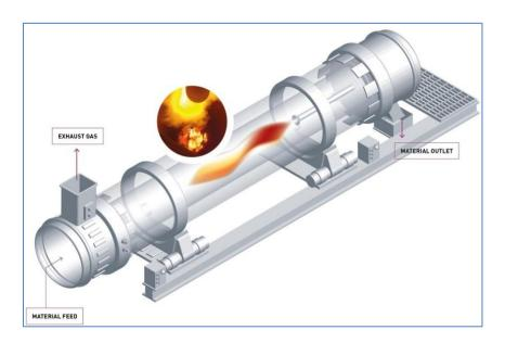
Figure I.11: Rotary kiln.
