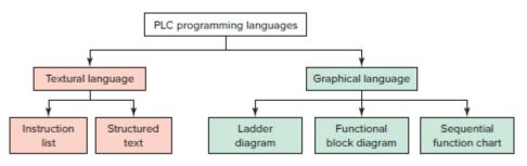
Figure II.11: Standard IEC 61131 languages associated with PLC programming.
