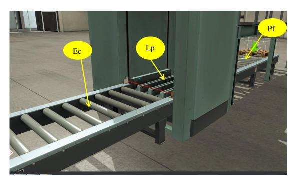
Figure III.5:Position of the actuators in the palletizer at the bottom.
