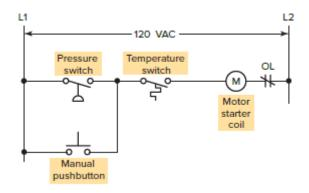
Figure II.9: Relay ladder diagram for the modified process.
