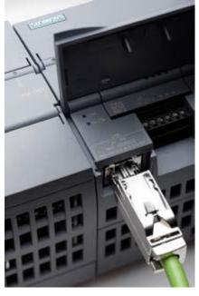
Figure II.18: PROFINET connection.
