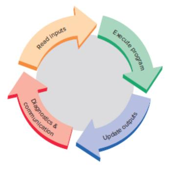
Figure II.8: Typical PLC scan cycle.
