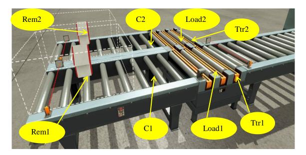
Figure III.8: Position of the actuators in the Chain Transfer.
