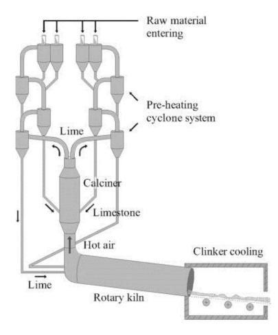
Figure I.9: Production stages of clinker.
