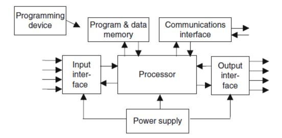
Figure II.7: The PLC system.
