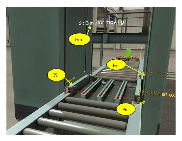
Figure III.3: Position of the sensors in the palletizer at the bottom.
