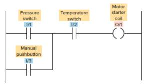
Figure II.10: PLC ladder logic program for the modified process.
