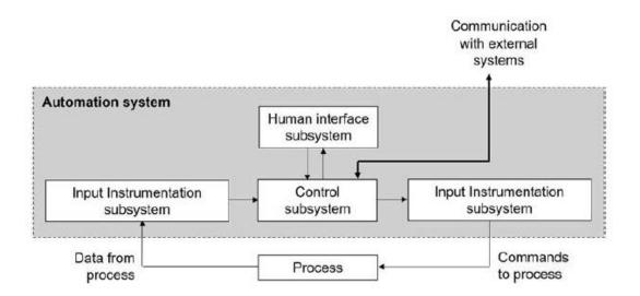
Figure I.16: Basic structure of automation system.
