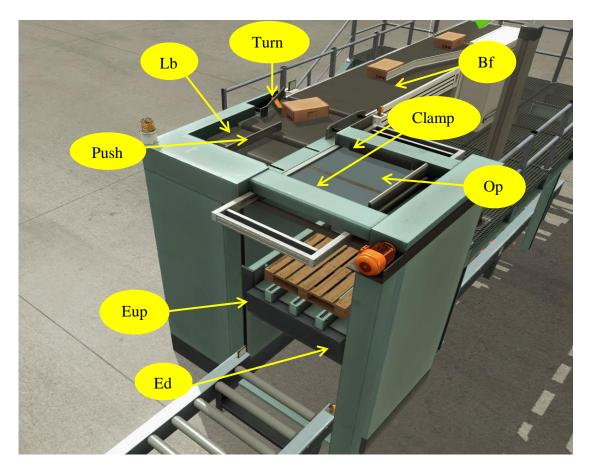
Figure III.6 Position of the actuators in the palletizer at the top.
