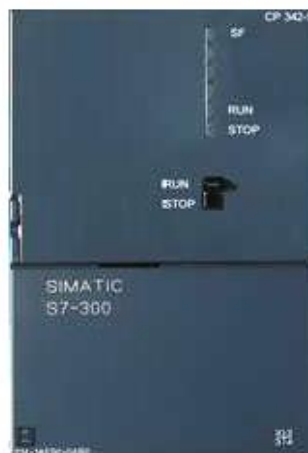
Figure 2.7: Modules de communication (CP) [11].
