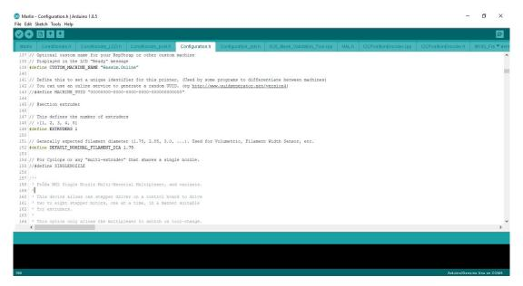
Figure 2.16: Default Nominal Filament Diameter
