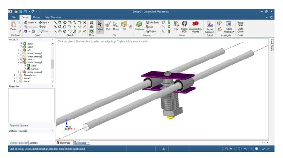
Figure 3.38: 3D design of X axis movement components
