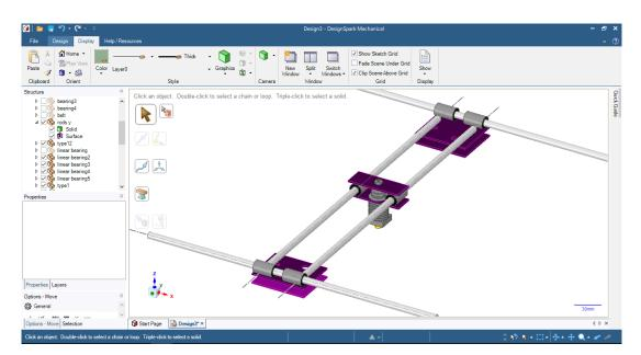
Figure 3.39: 3D design of X and Y axis movement components
