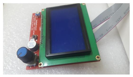
Figure 3.8: 3D Printer LCD display controller
