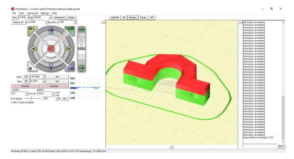
Figure 4.44: near finish printing progress as shown on Pronterface
