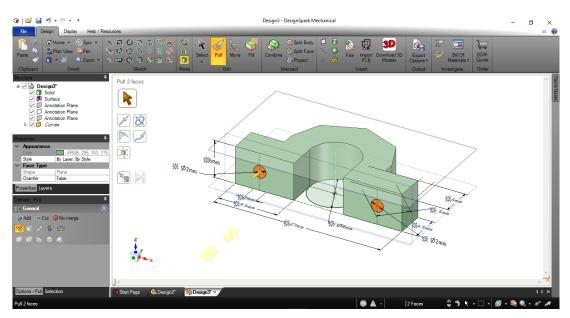
Figure 4.28: making holes for the end-stop holder
