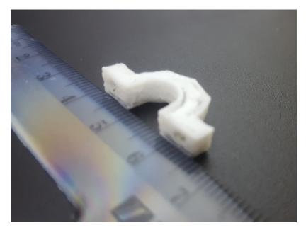
Figure 4.46: end-stop holder dimension accuracy check
