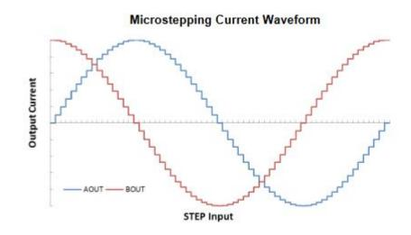
Figure 3.17: Stepper driver micro-stepping current waveform [TI11]
