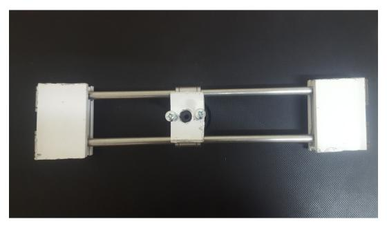
Figure 4.13: top view of the X axis movement components assembled
