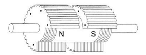
Figure 2.2: Hybrid stepper motor rotor
