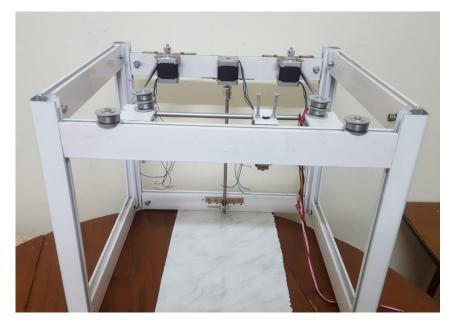
Figure 4.17: 3D printer view before mounting the printing base
