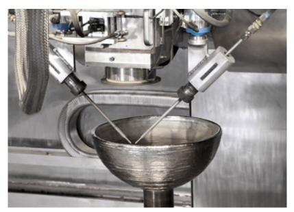
Figure 1.14: Electron Beam Melting [typ18]
