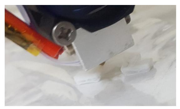
Figure 4.43: during end-stop holder 3D printing process
