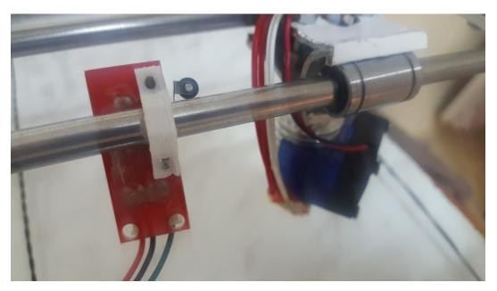
Figure 4.48: after using the 3D printed end-stop holder
