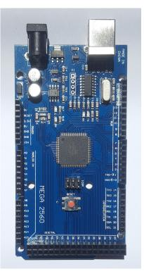
Figure 3.10: Picture of the ARDUINO mega board
