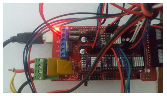
Figure 4.20: Wiring of the 3D printer electronic components
