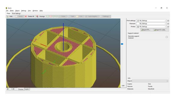
Figure 4.7: Slicing the 3d model using Slic3r
