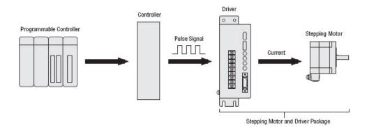
Figure 2.3: Stepper motor control
