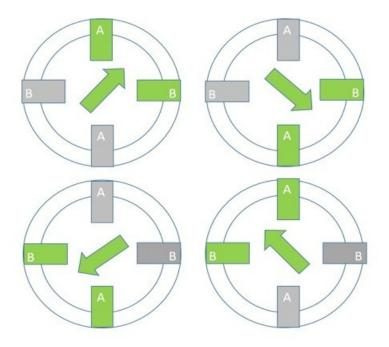
Figure 2.10: Two phase on, Full step
