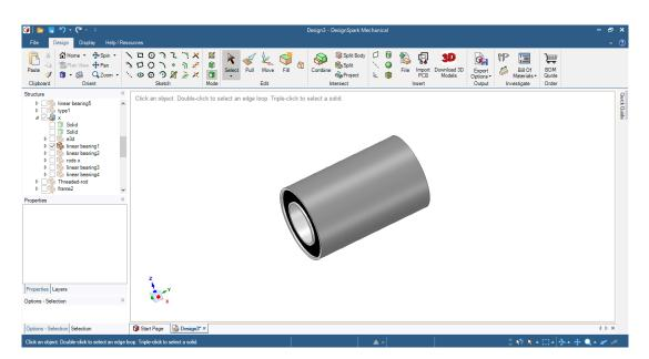
Figure 3.33: 3D design of a linear bearing
