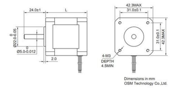
Figure 3.3: Dimensions of NEMA 17 stepper motor[dim]
