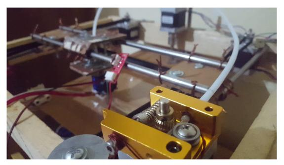
Figure 4.4: After mounting the extruder
