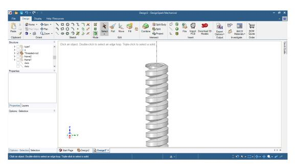
Figure 3.37: 3D design of a threaded rod
