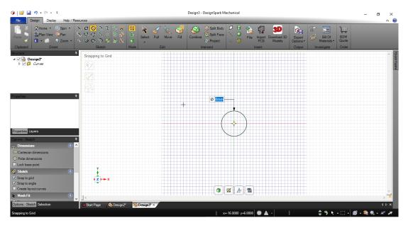
Figure 4.23: sketching circle 8 mm diameter
