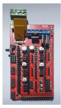
Figure 3.12: Picture of The RAMPS board
