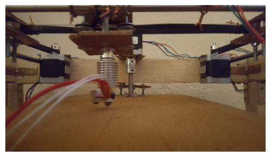
Figure 4.3: After mounting the base and the z axis
