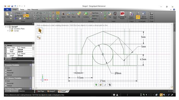
Figure 4.26: final geometry of the end-stop holder with lengths
