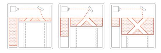
Figure 1.8: 3D printing process Powder Bed Fusion (Polymers) based [All19]
