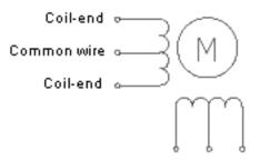
Figure 3.1: Unipolar stepper motor coils
