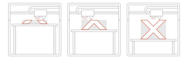
Figure 1.10: 3D printing process Material Jetting based [All19]
