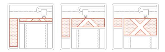
Figure 1.12: 3D printing process Binder Jetting based [All19]
