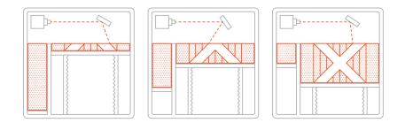
Figure 1.13: 3D printing process Powder Bed Fusion (Metals) based [All19]
