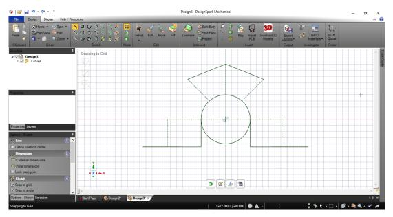
Figure 4.25: sketching the geometry of the end-stop holder
