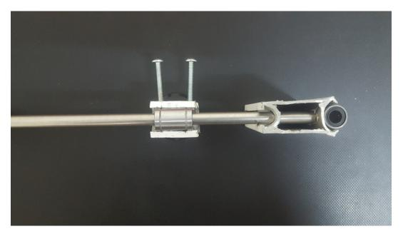
Figure 4.14: side view of the X axis movement components assembled
