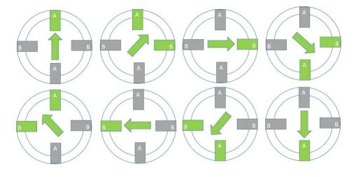
Figure 2.11: One-Two phase on, Half step
