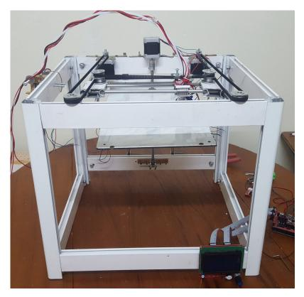
Figure 4.19: 3D printer view after mounting the printing base
