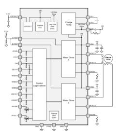
Figure 3.15: functional block diagram of the stepper driver [TI11]
