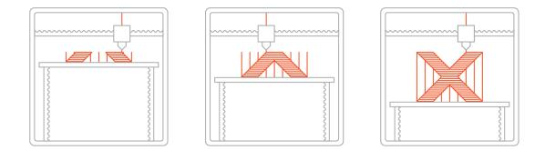
Figure 1.2: 3D Printing Process Material Extrusion based [All19]
