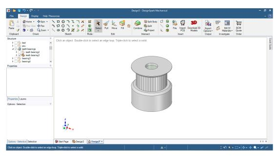
Figure 3.36: 3D design of the of timing belt pulley
