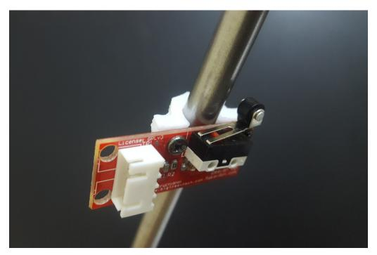
Figure 4.49: utilizing the 3D printed end-stop holder
