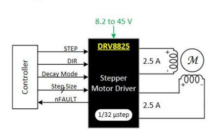
Figure 3.14: Stepper driver simplified schematics [TI11]
