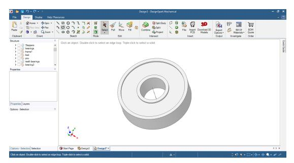
Figure 3.34: 3D design of a ball bearing
