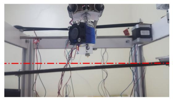
Figure 4.21: Tilted printing base side view
