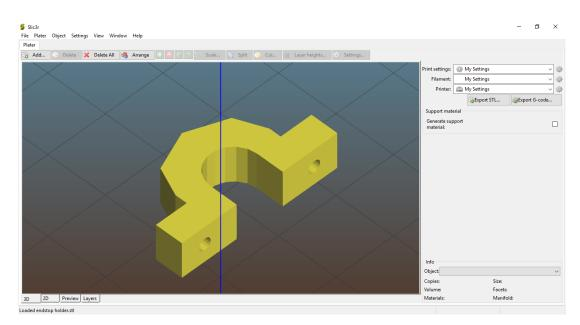
Figure 4.31: importing the model to Slic3r
