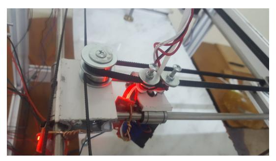
Figure 4.41: End-stops indicating home position at X0 Y0
