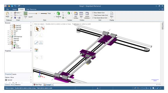
Figure 3.40: Bearings and belt installation
