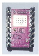
Figure 3.16: stepper driver back view
