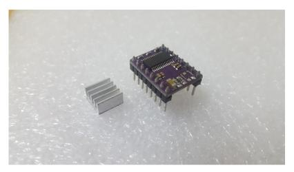
Figure 3.13: stepper driver drv8825 with heat-sink
