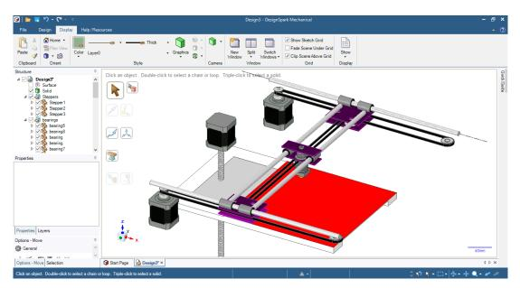
Figure 3.42: Initial concept of the 3D printer without frame
