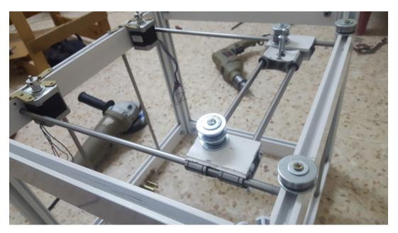
Figure 4.15: X and Y movement components
