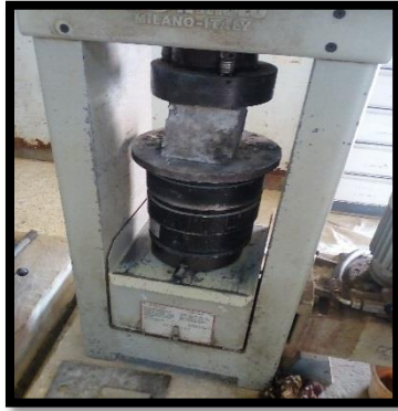
Photo III.4: Machine Essai de Compression
