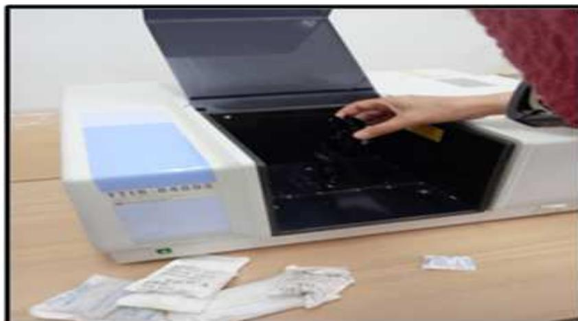
**Figure II. 14 :** Appareil FT-IR.
