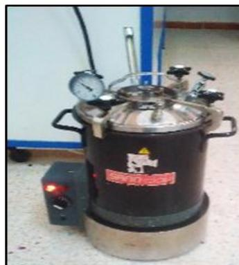
**Figure III.5 :** Autoclave.
