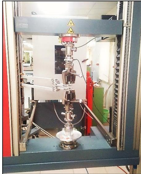
**Figure III.4 :** Machine de traction.
