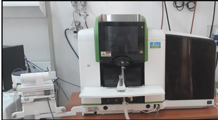
Figure 36 :PinAAcle 900T Atomic Absorption Spectrometer(2019)
