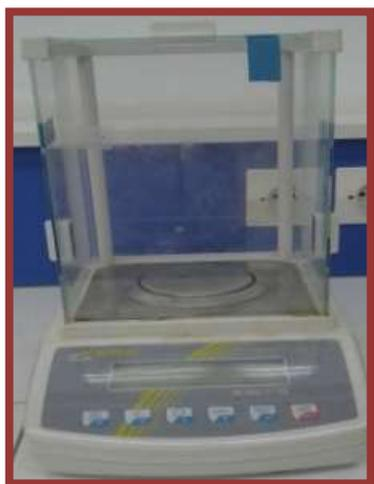
**Figure (II.8):** digital scale.
