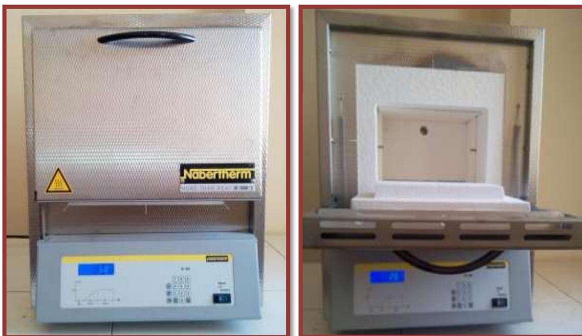
**Figure (II.13):** The annealing furnace.
