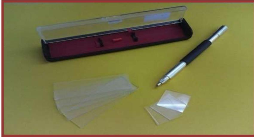
**Figure (II.6) : Substrates cut .**
