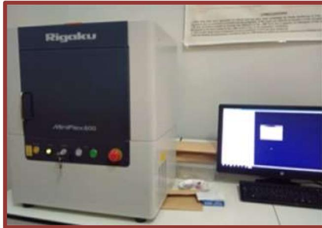
**Figure (II.16):** The x-ray diffractometer used in the analysis of x-ray diffraction of the samples.
