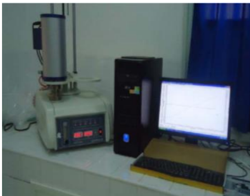
Figure II.6 : Appareil ATD-ATG de marque LINSEIS STA 2400.
