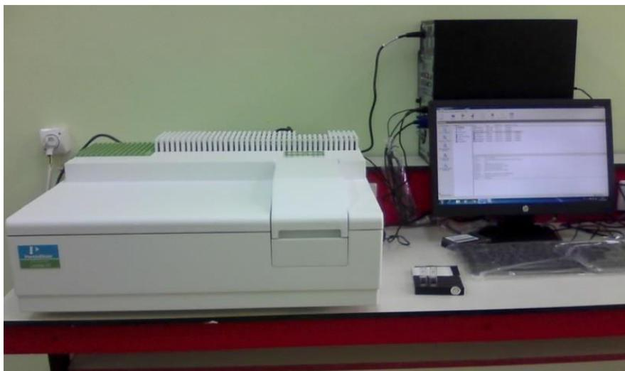
**Figure II.3.6:** spectrométrie UV-visible type "Perkin Elmer Lambda 25 UV.
