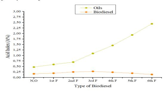
Figure IV.10: Evolution of the acid index of oils and biodiesels
