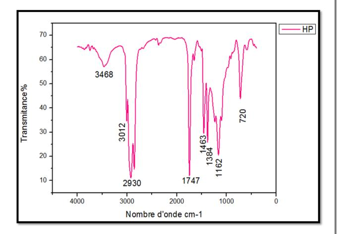
Figure IV.1: Spectrum of FT-IR for new oil with brand Elio
