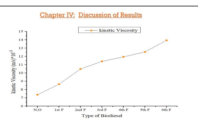
Figure IV.8: The graph curve represents viscosity in term of speed changes with different type of biodiesel
