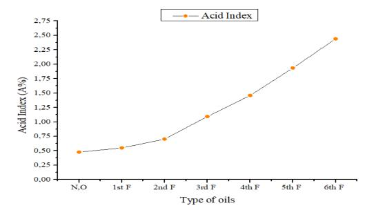
Figure IV.2: The graph curve represents Acid index changes with different type of oils
