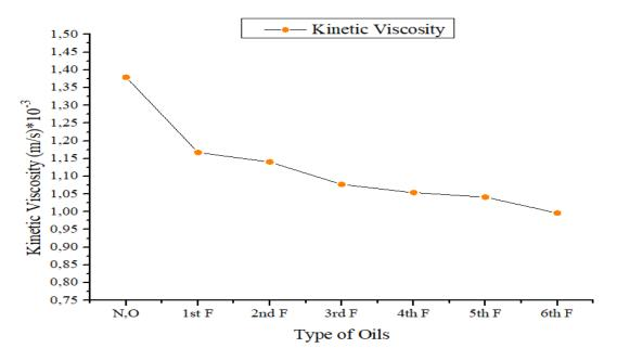
Figure IV.4: The graph curve represents viscosity in term of speed changes with different type of oils
