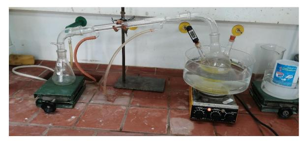
Figure III.13: Experimental example of distillation process with Biodiesel 5<sup>th</sup> frying oil
