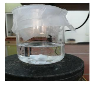
Figure III.9: The mixture of methanol and Catalyst KOH
