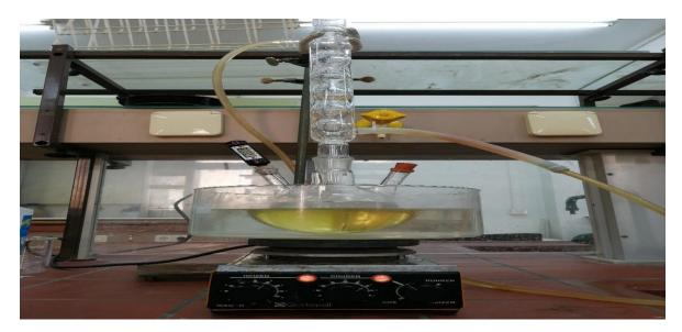
Figure III.10: Experimental example of process heating circuit with mixture of new oil with methanol.
