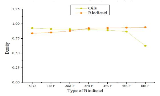
Figure IV.11: Evolution of the density index of oils and biodiesels
