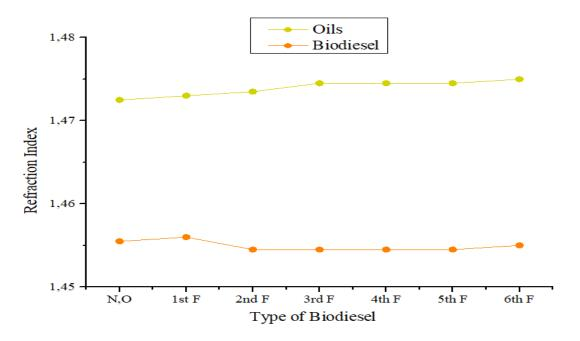
Figure IV.13: Evolution of the refraction index of oils and biodiesels
