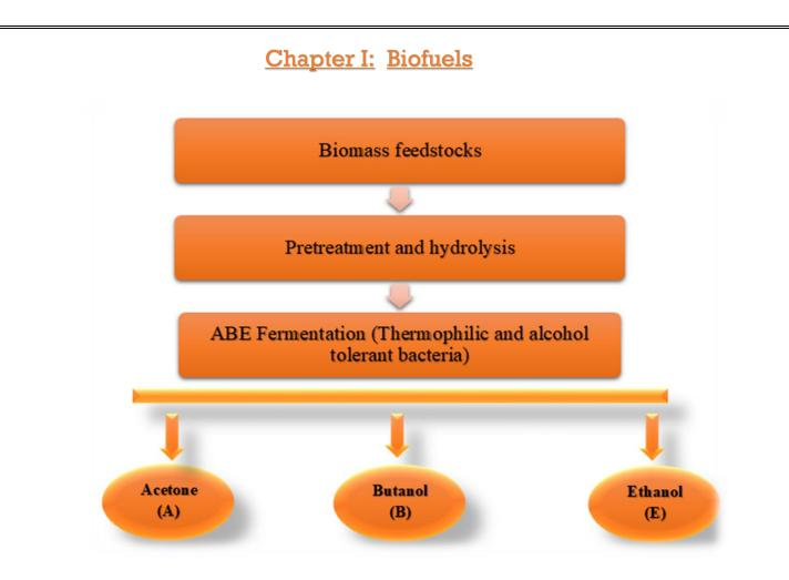
Figure I.6: A general schematic of biobutanol production via ABE fermentation.
