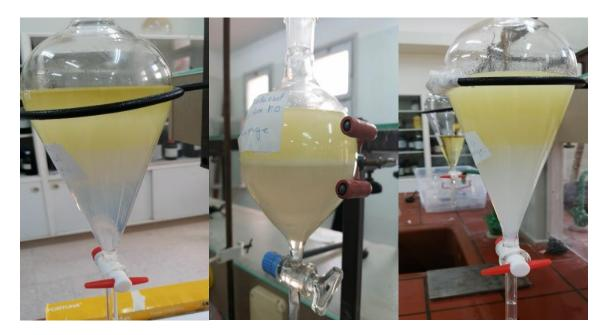
Figure III.12: Experimental examples of washing up step with biodiesel new oil, biodiesel 3<sup>rd</sup> frying oil and biodiesel 6<sup>th</sup> frying oil
