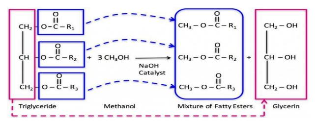
Figure III.8: Chemistry of Biodiesel production.
