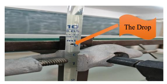
Figure III.5: An experimental example for measuring viscosity of New Oil.
