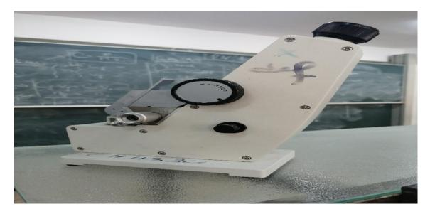
Figure III.3: Refractometer used {Princeton instruments, model 24AJ, serial}.
