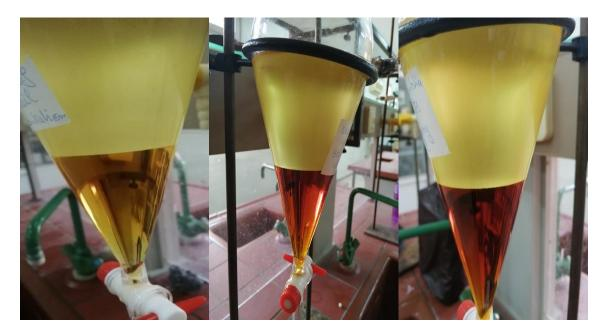
**Figure III.11:** Experimental examples of decantation step with new oil, 3<sup>rd</sup> frying oil and 6<sup>th</sup> frying oil.
