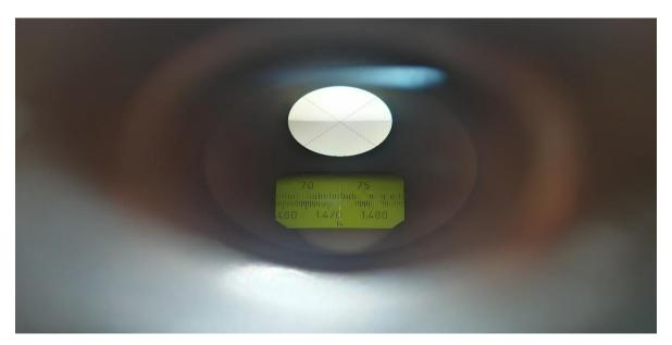
Figure III.4: An experimental example for measuring refraction index for new oil.
