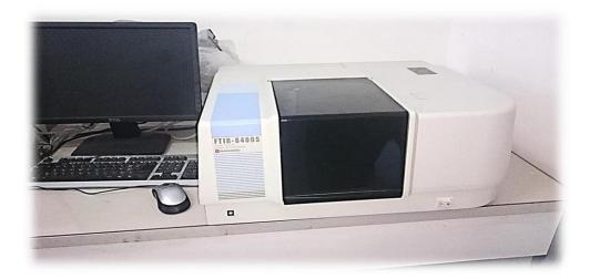
Figure I.8.IR spectroscopy dispositive.
