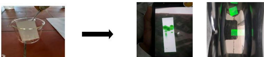
Figure III.16 : CCM de la chalcone
