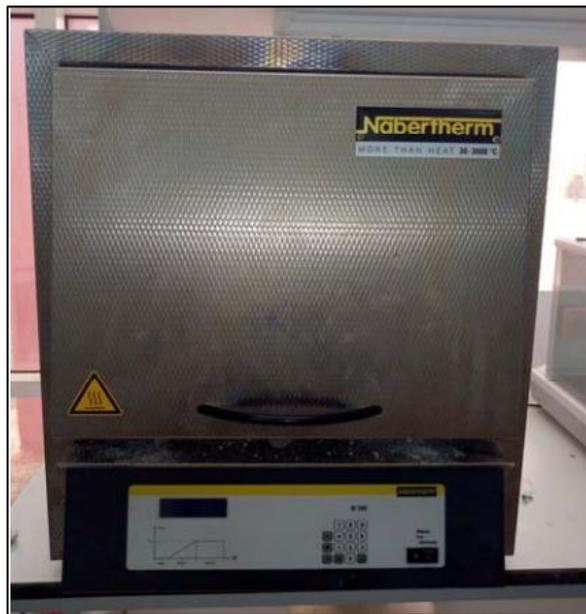
**Figure II .4:** Four Nabertherm  $1250^{\circ}\text{C}$ .
