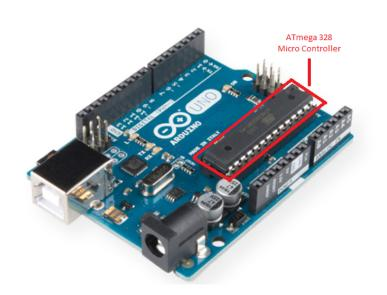
Figure 5: Labelled Arduino board.
