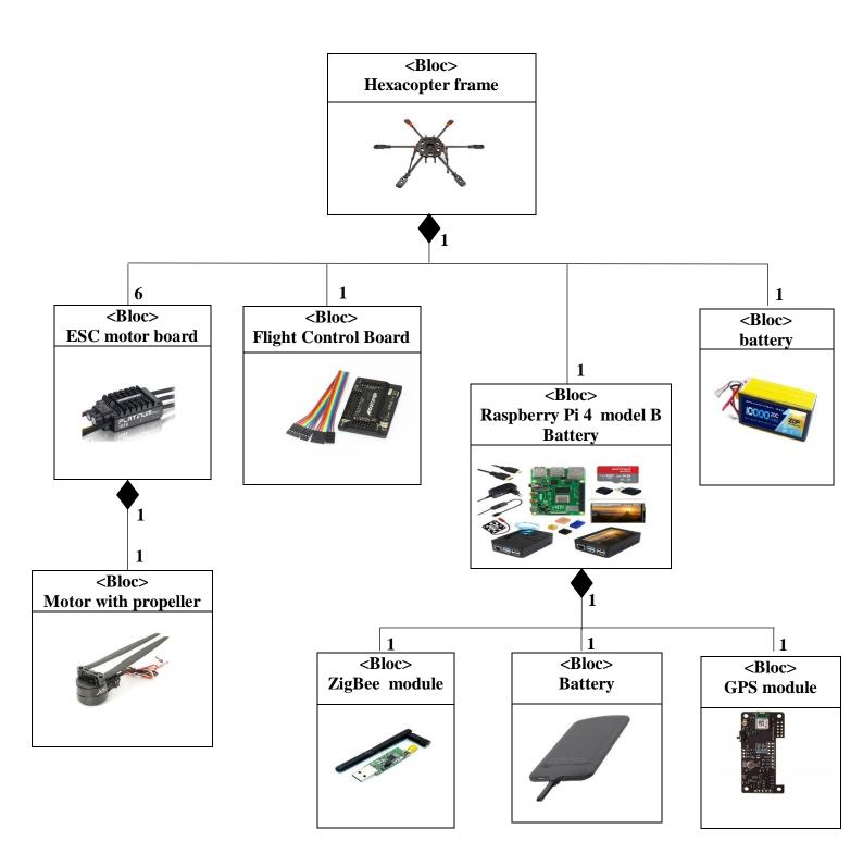
Figure 3. 3: The hardware architecture of the UAV Broker.
