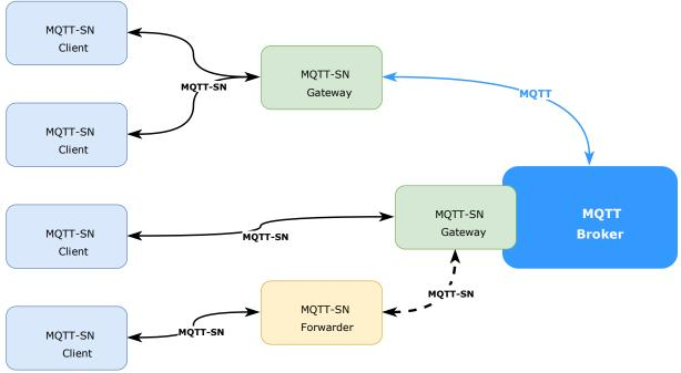
Figure 2. 7: MQTT-SN architecture. [24]
