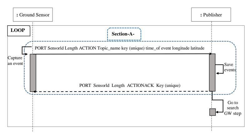
Figure 3. 5: Ground Sensor and Publisher sequence diagram.
