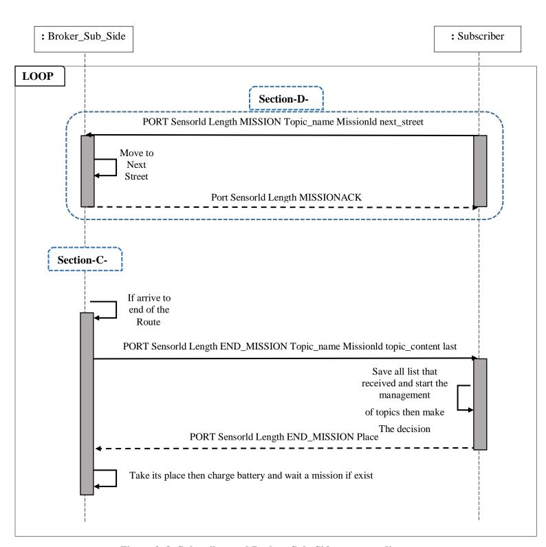
Figure 3. 8: Subscriber and Broker\_Sub\_Side sequence diagram.
