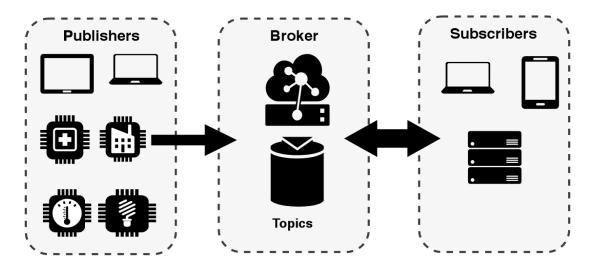
Figure 2. 3: MQTT architecture. [23]
