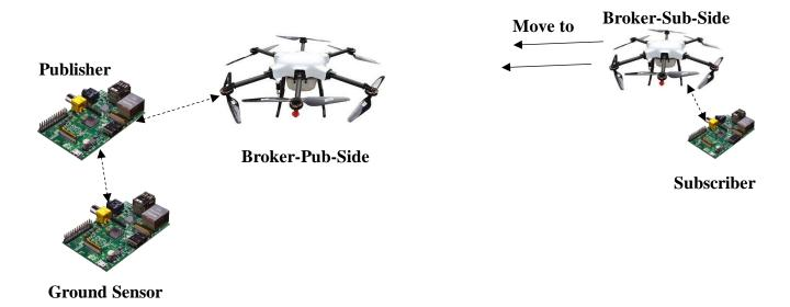
Figure 3. 4: publish /subscribe Architecture based UAV Brokers.
