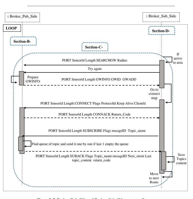
Figure 3. 7: Broker\_Pub\_Side and Broker\_Sub\_Side sequence diagram.
