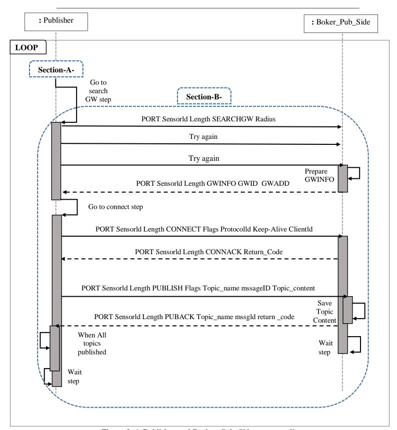
Figure 3. 6: Publisher and Broker\_Sub\_Side sequence diagram.
