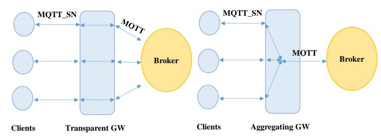
Figure 2. 8: The Transparent and Aggregating. [24]
