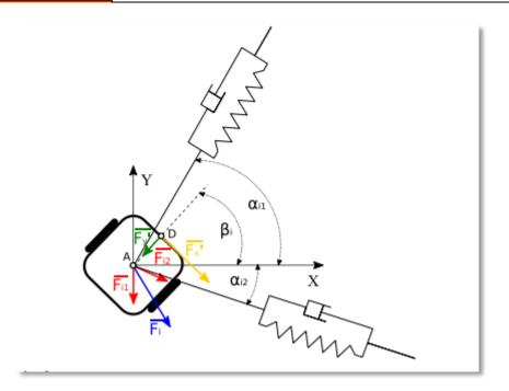
Figure. 3.5 Robot i driving forces
