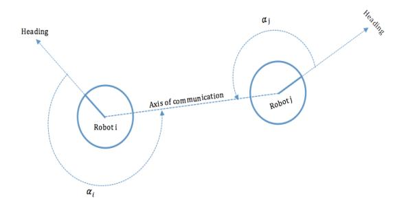
FIGURE 2.6: The relative position measurements within the communication system.[17]
