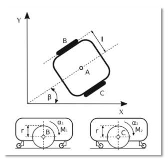
Figure. 3.2 Two-wheel robot schematic [24, 25]
