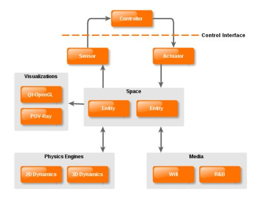
Figure 4.1 The general architecture of ARGoS [22]
