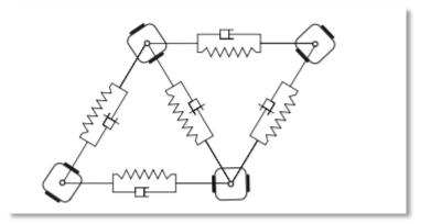
Figure. 3.3 Spring dampers mesh connecting mobile robots
