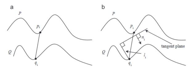
Figure 2.17: (a) Point to point error metric (b) point to tangent plane error metric.
