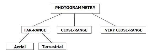
Figure 2.4: Classification of Photogrammetry methods [45].
