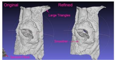
Figure 2.15: Mesh Filtering Node [60].
