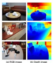
Figure 4.15. An example of with image RGB-D Captured for a camera Kinect.
