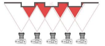
Figure 2.6: Image acquisition method for large objects' reconstruction [43].
