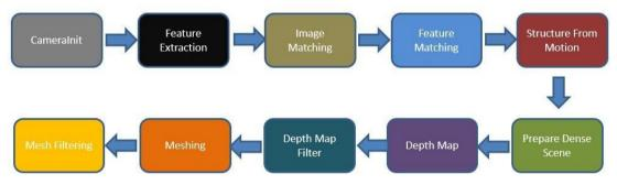
Figure 2.11: Meshroom Photogrammetry Pipeline.
