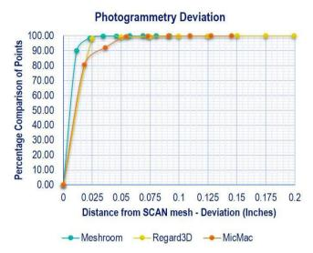
Figure 2.10: Comparison of c2c deviation of photogrammetry tools.
