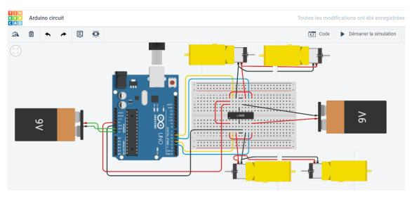
Figure 4.20 – Hardware system design
