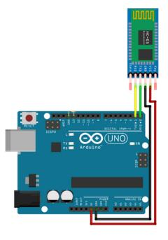
Figure 4.27 - Hc05 connection to Arduino
