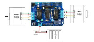
Figure 4.23 – Design motor, power and driver sheild wires connection
