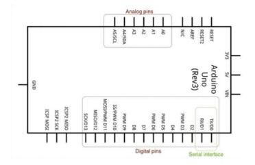
Figure 4.15 – The pins on uno board
