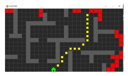
Figure 3.7 – Path from home to cross icon in djikstra algorithm
