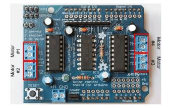
Figure 4.13 – Place of each motor
