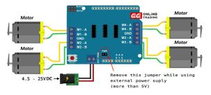
Figure 4.22 – Motor, power and driver sheild wires connection
