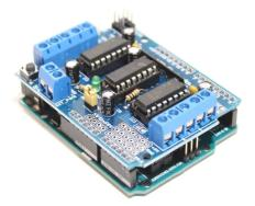
Figure 4.18 – L293D Motor Driver Shield
