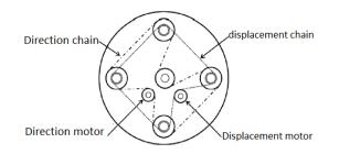
Figure 2.11 – Synchronous traction configuration
