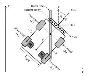
Figure 2.7 – Configuration of a mobile to differential drive
