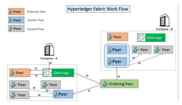
Figure 1.16: HyperLedger Fabric Transaction Flow [23].
