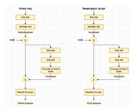
Figure 1.11: Calculate of Bitcoin Address [103].
