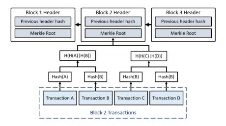
Figure 1.10: The architecture of Merkle tree in the blockchain [72].
