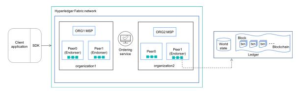
Figure 1.14: The components of a Hyperledger Fabric network [91].
