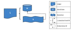
Figure 1.15: Ledger consists of W-World State and B-Blockchain [26].
