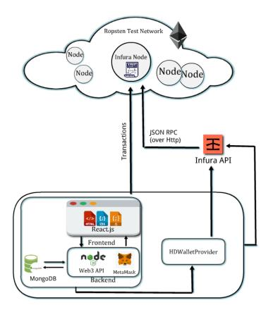
Figure 3.2: Detailed Architecture of The System
