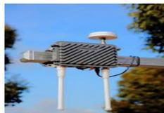
FIGURE 2.3 – Road Side Unit (RSU)
