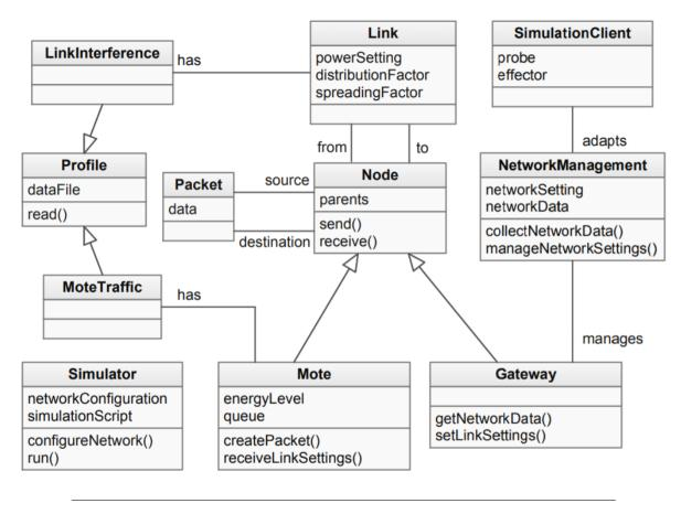
FIGURE 5.1: Architecture of DeltaIoT Simulator [39].
