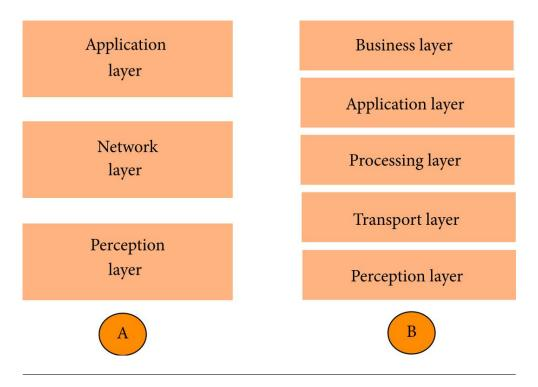
FIGURE 1.1: Architecture of IoT (A: three layers) (B: five layers). [2].
