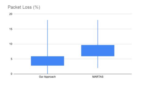
FIGURE 5.15: Test results for Our Approach versus MARTAS in Packet loss.
