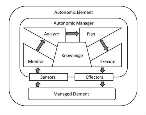
FIGURE 2.2: The IBM reference model for autonomic computing MAPE-K.
