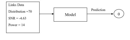
FIGURE 4.4: Example of the prediction process of Packet Loss.
