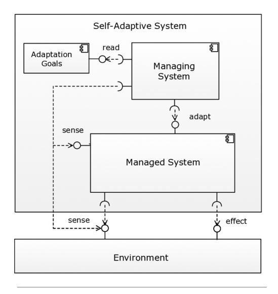
FIGURE 2.1: Conceptual model of a self-adaptive system. [10]
