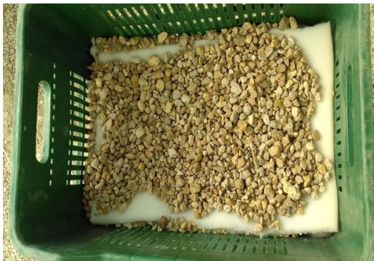
Figure 07 : caisse de filtration (Original)
