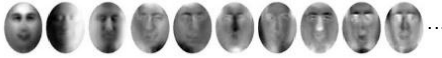
Figure 2.10: The measurement mode matrix U_x contains the conventional PCA eigenvectors (“eigen-faces”), which are the principal axes of variation across all the images. The first 10 eigenvectors are shown.
