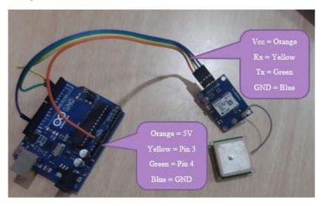
Figure III. 12 GPS with Arduino in Real
