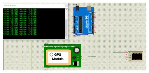
Figure III. 14the results of GPS and ARDUINO UNO
