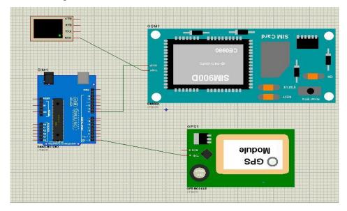
Figure III. 15GPS Tracker circuit in PROTEUS
