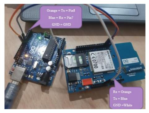
Figure III. 10GSM with Arduino in Real
