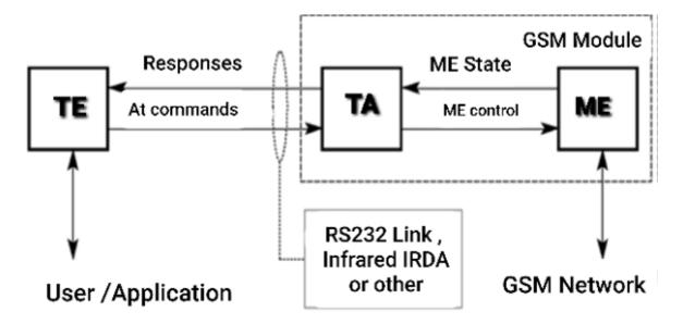
Figure II.10 diagram of the operation of AT commands [44].
