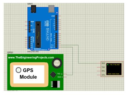
Figure III. 11 GPS and ARDUINO UNO circuit in PROTEUS
