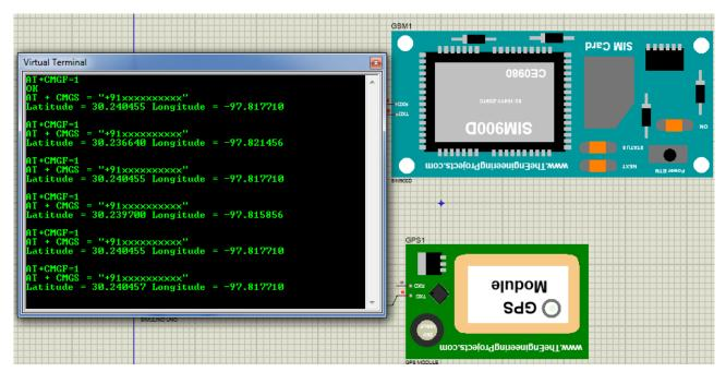
Figure III. 18the Result of GPS Tracker
