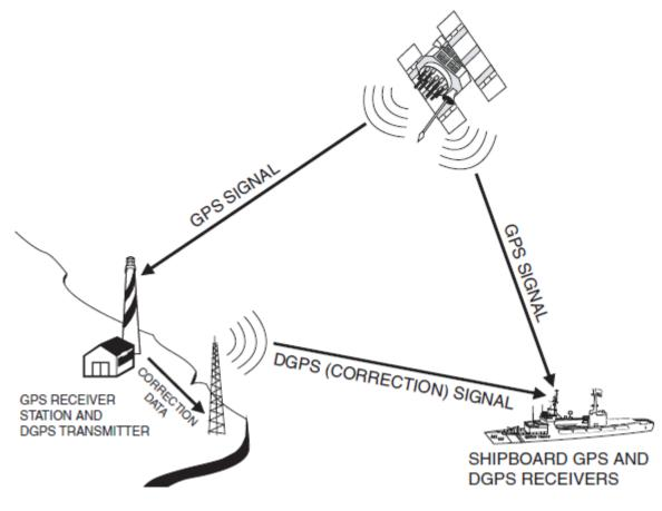
Figure I.7How DGPS works[5].
