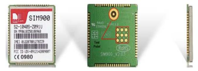
Figure II. 8top, bottom side view of sim900 [43].
