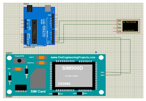
Figure III. 9GSM and ARDUINO UNO circuit in PROTEUS
