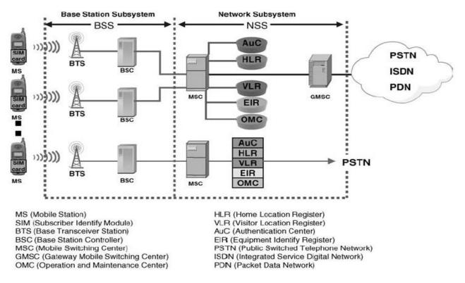
Figure II. 1 GSM System Architecture [23].
