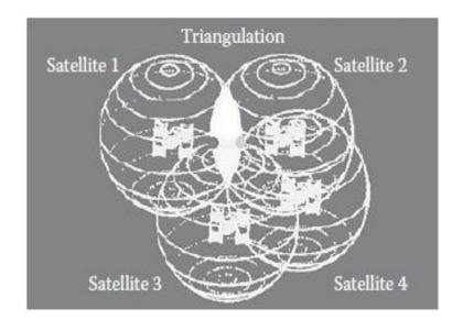
Figure I.1 Basic principle of positioning with GPS [4]
