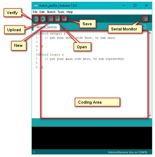
Figure III. 2Interface of Arduino IDE
