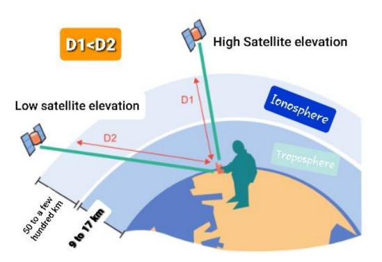
Figure I.4Sources of error due to atmospheric effects [13].
