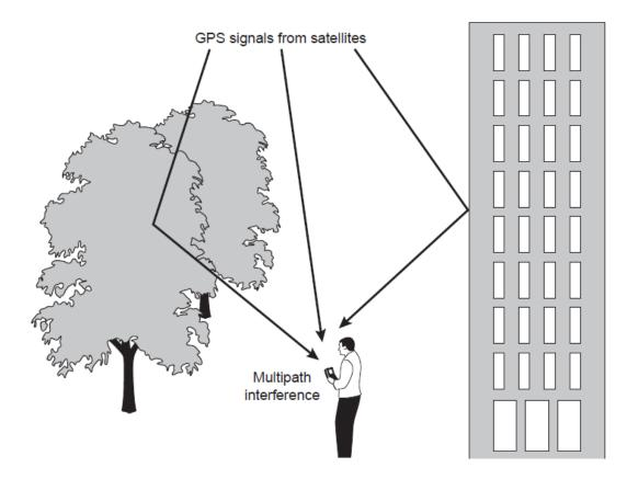
Figure I.5Effects of buildings and solid objects on the satellite signals[15].
