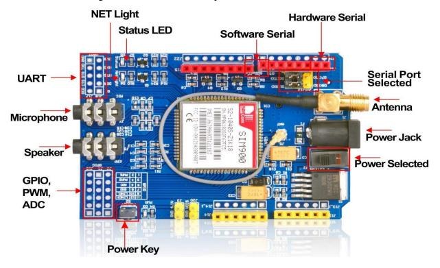
Figure II.7Description of the module GSM/GPRS Shield [40].
