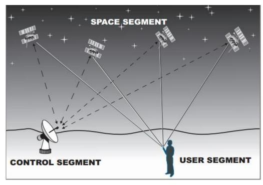
Figure I.2 The three segments of GPS [5]^
