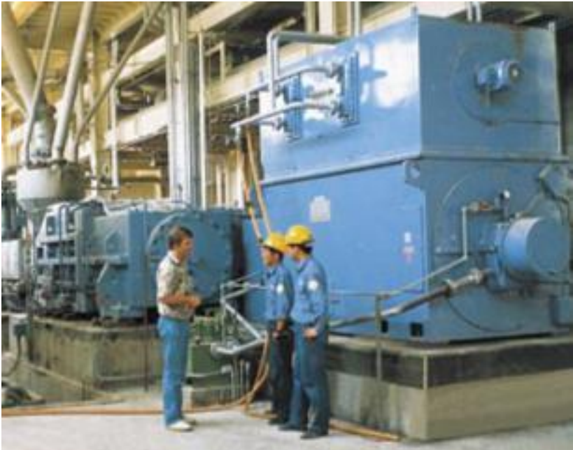
Figure II-3 :Polyethylene extruder drive with MEGADRIVE-LCI
