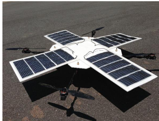
Figure I_25: drone uses solar cells.
