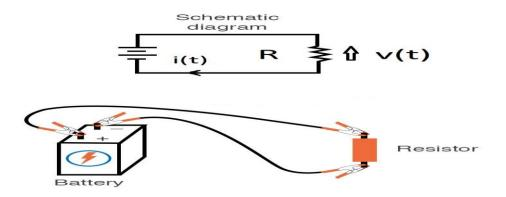
Figure I.2: Pure electrical resistance
