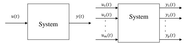
Figure I.7: Monovariable system (left), multivariable system (right).
