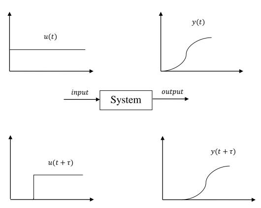
Figure I.6: Behavior of an invariant system
