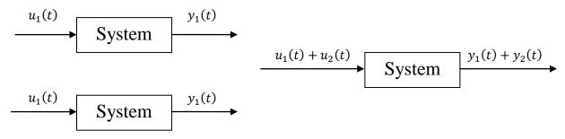
Figure I.5: Principle of superposition.
