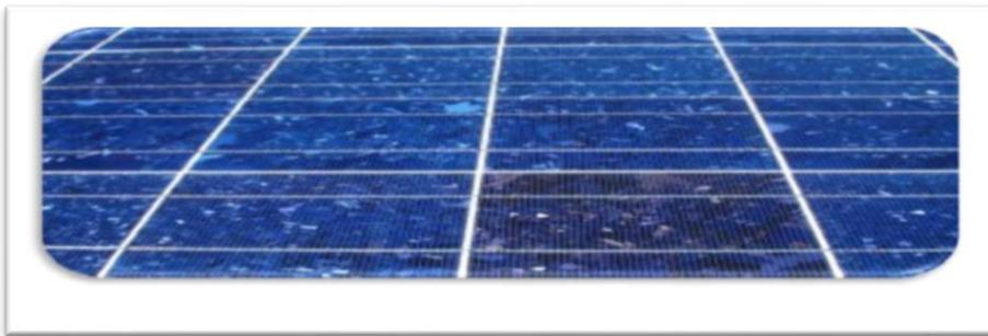
**Fig.I.5** Cellules photovoltaïques poly-cristallin [8].
