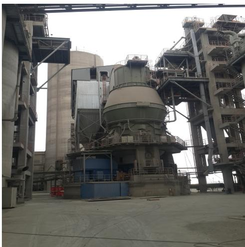
FIGURE 1.13 – Broyeur ciment vertical [1].
