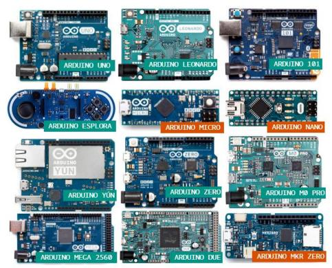
Figure II.1. The different Arduino boards [13].
