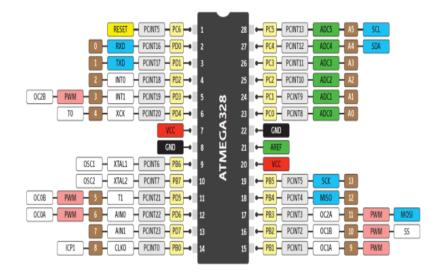
Figure II.3. The atmega328 microcontroller [16]
