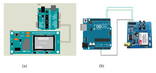
Figure III.21.Interfacing GSM with Arduino. (a) Proteus (b) on the Arduino board.
