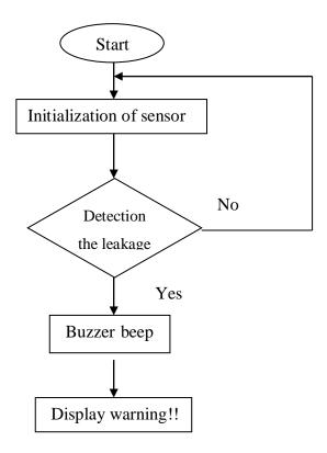
Figure III.19. flow chart of MQ-2 sensor.
