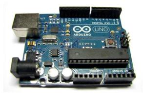
Figure II.2.Arduino Uno Board[14]
