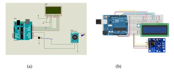
Figure III.18. Interfacing MQ-2 sensor with Arduino. (a) Proteus (b) on the Arduino board.
