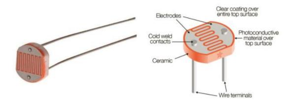
Figure II.10. Light Detecting Resistors (LDR) [35]
