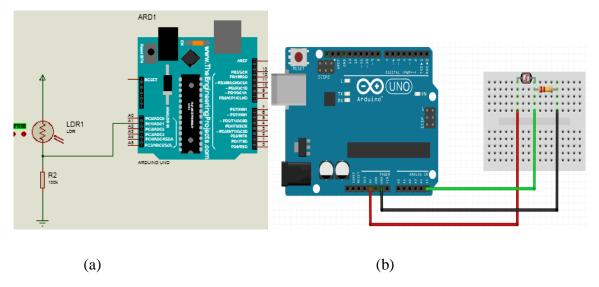
Figure III.22.Interfacing LDR with Arduino. (a) Proteus (b) on the Arduino board
