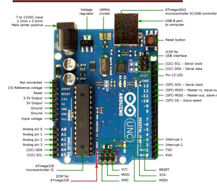
Figure II.4. Different parts of an Arduino [17]
