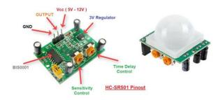
Figure II.6. PIR sensor [29]
