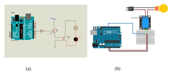
**III.5.4 Interfacing Relay with Arduino (controlling bulb)**
