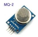
Figure II.5.MQ-2 gas detector [25]
