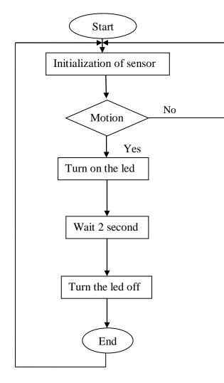
Figure III.17.flow chart of PIR sensor.
