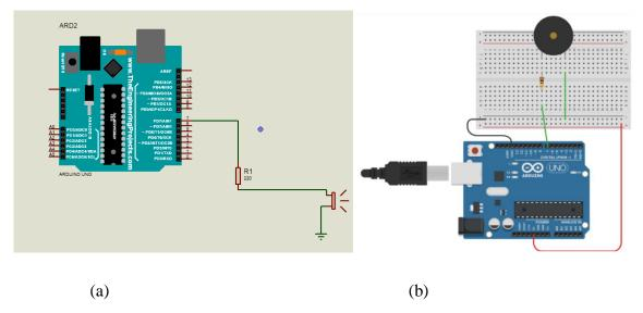
Figure III.23.Interfacing Buzzer with Arduino. (a) Proteus (b) on the Arduino board.
